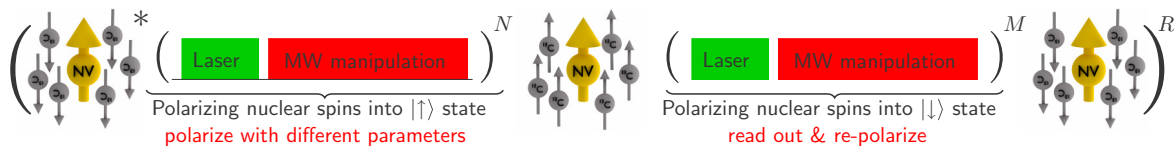
FIG. 1. Schematic representation of the experiments. The first pulse sequence is repeated N times and is used to polarize the nuclear spin bath along the static magnetic field ( |\uparrow\uparrow\uparrow\dots\rangle state). By changing the MW manipulation, we can polarize the nuclear spin bath into the |\downarrow\downarrow\downarrow\dots\rangle state by repeating the sequence M times. The illustrations present the state of the spin bath around the NV center at different time instants. At the beginning the nuclear spins are polarized in the |\downarrow\rangle state. After repeating the polarization sequence N times the nuclear spins are partially or fully inverted into the |\uparrow\rangle state depending on N . By polarization of the nuclear spin bath during the M cycles the nuclear spin bath is both initialized and read out. Hence, M has to be set large enough, so that the nuclear spin bath is completely polarized. At the start of the experiment at N, R = 1 (*) the nuclear spin bath is unpolarized, but due to a larger number of repetitions of the measurements ( R = 5 \times 10^4 ) the first iteration can be neglected. For most of our experiments N = 50 and M = 200 . See text for more details.
