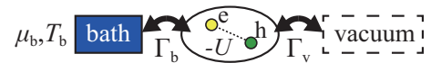
FIG. 2. Model driven-dissipative electron-hole gas. An electron-hole system with an attractive interaction -U is coupled to a pumping bath with the transfer matrix element \Gamma_b , as well as a vacuum with the transfer matrix element \Gamma_v . The pumping bath is assumed to be in an equilibrium state at the temperature T_b , where the particle distribution obeys the Fermi distribution function f_b(\omega) = 1/[e^{(\omega - \mu_b)/T_b} + 1] , where \mu_b is the chemical potential. The particle distribution f_v(\omega) in the vacuum vanishes.
