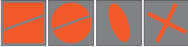
FIG. 7. Illustration of different conductor patch shapes on a grounded dielectric substrate for realizing an anisotropic tensor surface reactance. The solid gray square indicates the unit cell and the dielectric substrate. The conductor patch is shown in brown.
