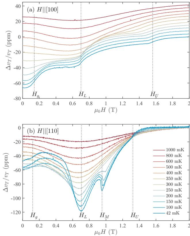
FIG. 1. Field scans of the relative change in transverse sound velocity  $\Delta v_T/v_T$  for various temperatures. The field is oriented along the [110] direction in (a) and along the [100] direction in (b). In (b) the curves are staggered for ease of view. The same legend applies to (a) and (b).
