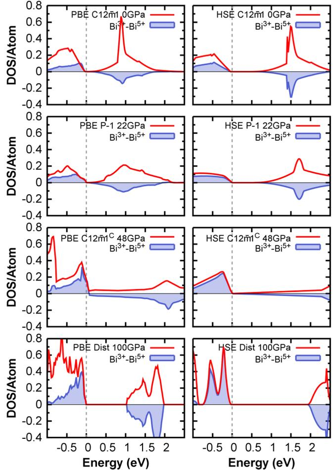
FIG. 5. DOS/atom and the difference of average PDOS for Bi<sup>5+</sup> and Bi<sup>3+</sup> atoms [69] for stable structures at the pressure of its stability. Left panel shows results obtained with PBE functional for structural relations and DOS calculations. Right panel shows results for structures at the left panel but DOS calculations were performed using the HSE functional using the structures from PBE calculations.
