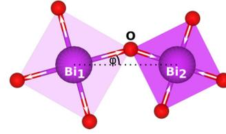
FIG. 3. Breathing and tilting distortions applied to an ideal cubic perovskite structure. Breathing is indicated by squares of different size where the white arrows show the direction in which O atoms are displaced. Tilting is shown as a rotation of a square by angle  $\varphi$  around axis normal to the plane of the paper.
