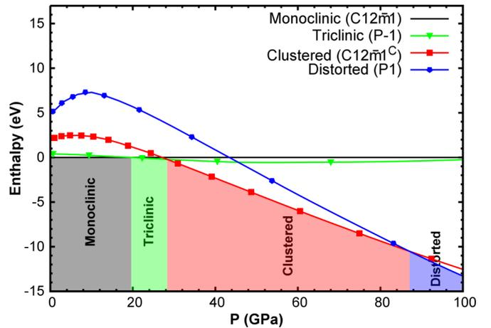
FIG. 2. Predicted high-pressure phase diagram of  $\text{BaBiO}_3$ . Up to 100 GPa, we predict three structural phase transitions: monoclinic ( $C12/\bar{m}1$ ) to triclinic ( $P\bar{1}$ ) at about 20 GPa, triclinic to clustered ( $C12/\bar{m}1^C$ ) at about 28 GPa, and clustered to distorted ( $P\bar{1}$ ) at about 87 GPa. The values of the enthalpies are referred to a 40 atoms unit cell.
