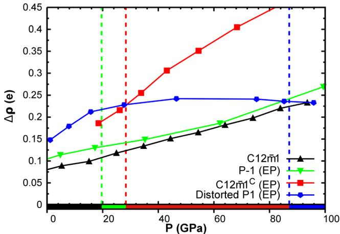
FIG. 6. Charge difference  $\Delta\rho$  between two different Bi atoms for all stable structures in the phase diagram: the one with the maximal charge (represented by the  $\text{Bi}^{3+}$  atom) and the one with the minimal (represented by the  $\text{Bi}^{5+}$  atom); the HSE functional was used. The color scale at the bottom indicates the stability range of the various structures.
