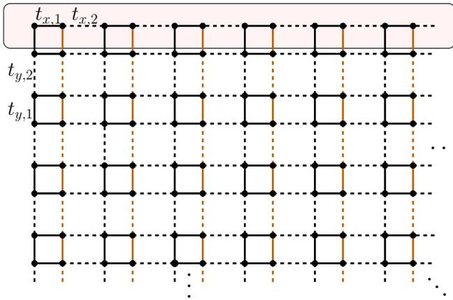
FIG. 2. Tight-binding model for a second-order topological insulator on a square lattice. Solid and dashed lines in the  $x$  and  $y$  directions denote alternating nearest-neighbor hoppings  $t_{x,1}$ ,  $t_{x,2}$  and  $t_{y,1}$ ,  $t_{y,2}$ . The hopping amplitudes for the bonds colored in brown include a relative minus sign. The effective Hamiltonian of the highlighted boundary parallel to the  $x$  direction is topologically equivalent to an SSH model.
