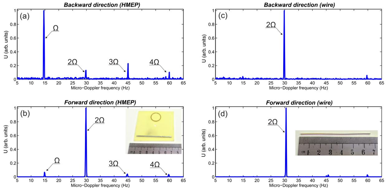
FIG. 6. Experimental observation of the micro-Doppler combs. (a) and (b) The HMEP particle, (c) and (d) the thin metal wire. Upper row is the backward direction, lower row is the forward direction. The angular frequency of mechanical rotation is  $\Omega = 2\pi \times 14$  Hz. The insets show photographs of the samples.
