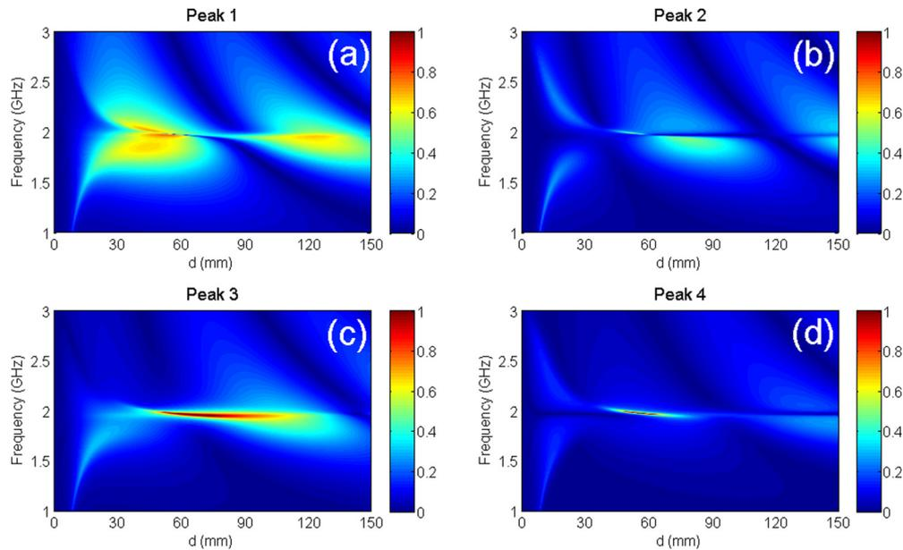
FIG. 4. Amplitudes of the micro-Doppler peaks in the backscattered signal from a HMEP as functions of the illumination frequency (vertical axis) and separation distance between the constitutive elements (horizontal axis): Color maps (a)–(d) refer, respectively, to the first, second, third, and fourth peak in the comb. All the amplitudes are normalized to the same value.
