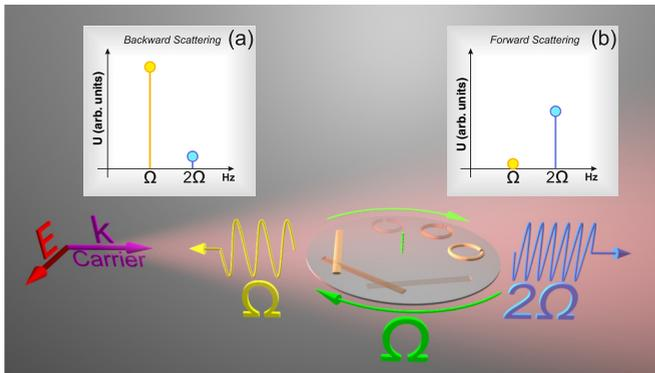
FIG. 1. Illustration of the generation of an asymmetric micro-Doppler comb by an axially rotating magnetoelectric particle (HMEP). The SRR and the wire constituting the HMEP are rotated with an angular frequency  $\Omega$  in the polarization plane of the incident wave. The forward and backward scattered fields demonstrate different micro-Doppler spectra (insets show frequencies at the baseband).
