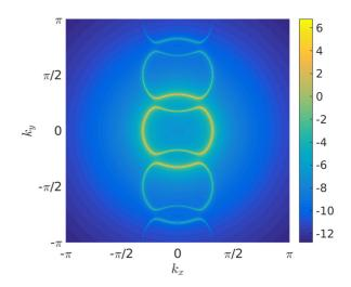
FIG. 4. The spectral function for a pair density wave state with wave vectors  $\pm Q = \pm (0, \pi/2)$ . The pockets are clearly visible.
