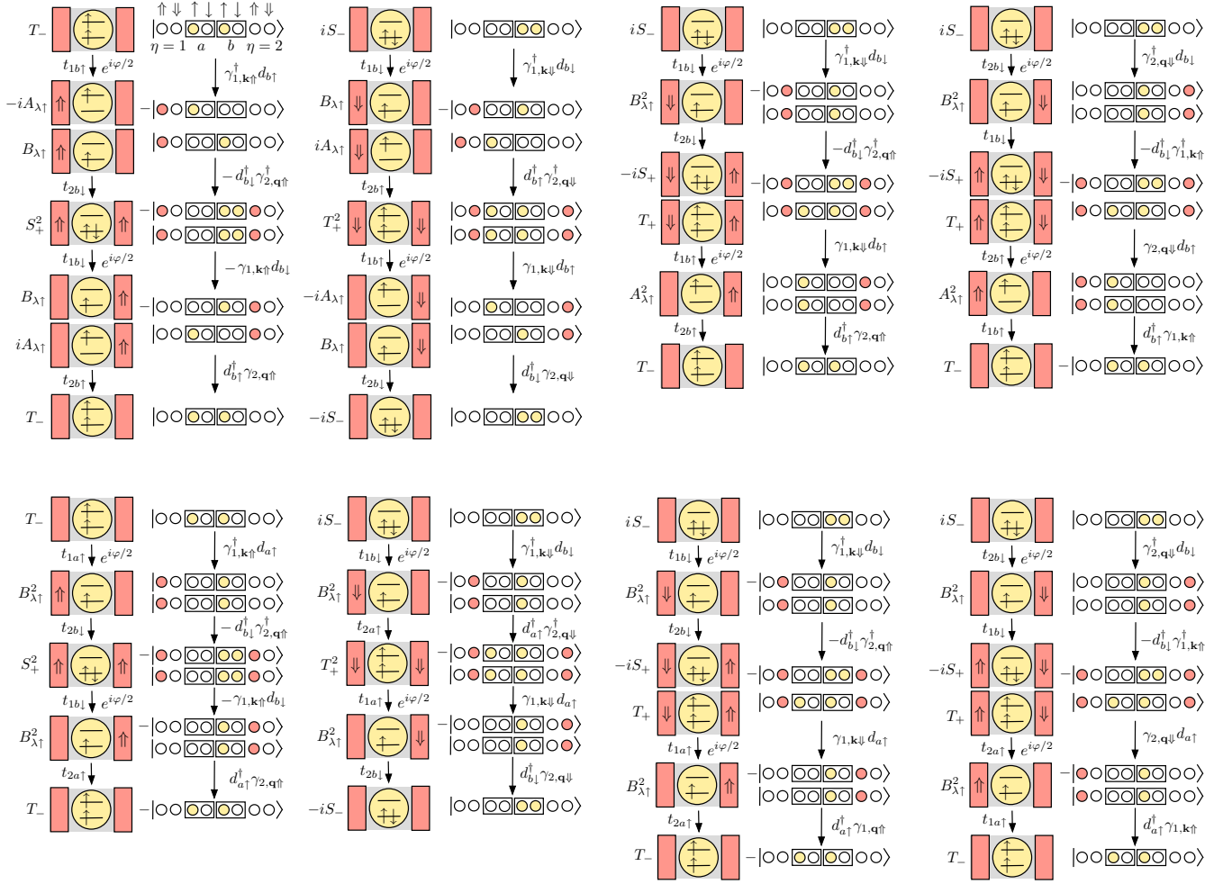
FIG. 3. Tunneling sequences (up to Hermitian conjugation) of the SC JJ for contributions \propto \cos \varphi_S . We use the basis |n_{1k\uparrow}, n_{1k\downarrow}, n_{a\uparrow}, n_{a\downarrow}, n_{b\uparrow}, n_{b\downarrow}, n_{2q\uparrow}, n_{2q\downarrow}\rangle = (\gamma_{1k\uparrow}^\dagger)^{n_{1k\uparrow}} (\gamma_{1k\downarrow}^\dagger)^{n_{1k\downarrow}} (d_{a\uparrow}^\dagger)^{n_{a\uparrow}} (d_{a\downarrow}^\dagger)^{n_{a\downarrow}} (d_{b\uparrow}^\dagger)^{n_{b\uparrow}} (d_{b\downarrow}^\dagger)^{n_{b\downarrow}} (\gamma_{2q\uparrow}^\dagger)^{n_{2q\uparrow}} (\gamma_{2q\downarrow}^\dagger)^{n_{2q\downarrow}} |0_1, 0_D, 0_2\rangle . Filled (empty) dots are used to visually represent a filled (empty) level.
