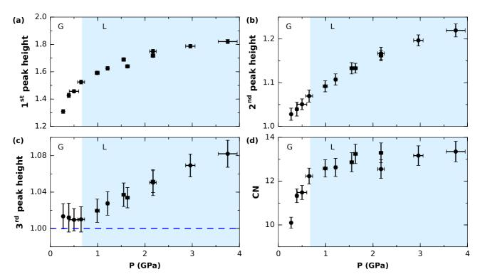
FIG. 3. Maxima of the first (a), second (b), and third (c) peak of the experimentally derived g(r) of neon against pressure. Error bars are calculated from the standard deviation of g(r) below the first peak. Dashed blue vertical line in (c) at 1 serves as a guide for the eye. Coordination number (CN) obtained by integrating g(r) up to the minimum after the first peak is shown in (d). The background shadings indicate the region for gaslike (G) and liquidlike (L) supercritical fluid.
