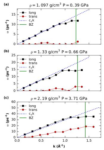
FIG. 6. Excitation spectra of neon derived from MD simulations at pressure points (a) above (b) nearly at and (c) below the Frenkel line. Longitudinal (squares) and transverse (circles) spectra are shown. The dashed lines give the Debye dispersion law  $\omega = c_s k$ , where  $c_s$  is the adiabatic speed of sound. The vertical lines mark the boundary of pseudo-Brillouin zone (BZ).
