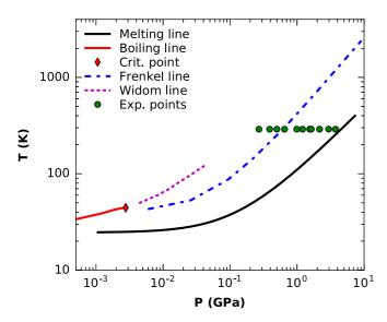
FIG. 5. The calculated Frenkel line for neon, shown together with the boiling line, melting line, Widom line (calculated from maximum of heat capacity taken from Ref. [35]), and experimental points in this study.
