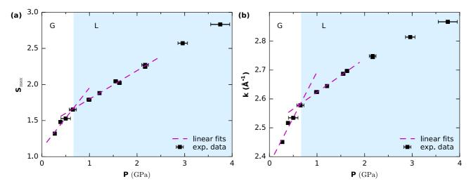
FIG. 2. Extracted height (a) and position (b) of the first maximum of the experimentally derived structure factor S(k) against pressure. The dashed magenta lines show the difference in slopes below and above the crossover. The background shadings indicate the region for gaslike (G) and liquidlike (L) supercritical fluid.
