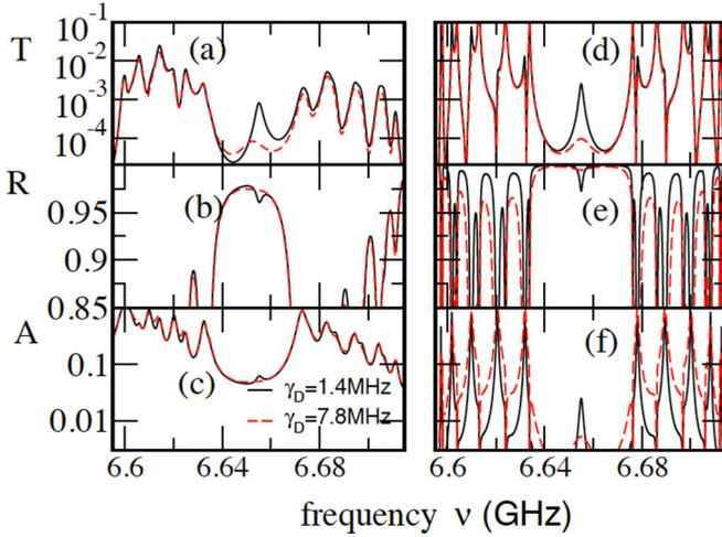
FIG. 2. Measurements of the (a) transmittance  $T$ , (b) reflectance  $R$ , and (c) absorption  $A$  for the C-CROW of Fig. 1. We considered two different values of  $\gamma_D = 1.4$  and  $7.8$  MHz. All other resonators have  $\gamma = 1.4$  MHz. Simulations for (d)  $T$ , (e)  $R$ , and (f)  $A$  of a C-CROW with lossless resonators ( $\gamma = 0$ ) apart from the defect resonator which has  $\gamma_D = 1.4$  MHz (solid lines) and  $\gamma_D = 7.8$  MHz (dashed lines).
