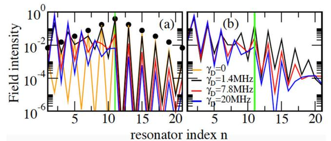
FIG. 4. (a) Simulations for an ideal C-CROW consisting of resonators with  $\gamma = 0$ . Solid black circles correspond to Eq. (2) for the defect mode profile. Solid lines correspond to the simulations of the resonant defect mode profile for various  $\gamma_D$ . For symmetry reasons we assumed that the antennas are coupled to the first and last resonator. (b) Experimental resonant mode profiles for various  $\gamma_D$  values. The measured losses at all resonators are  $\gamma = 1.4$  MHz.
