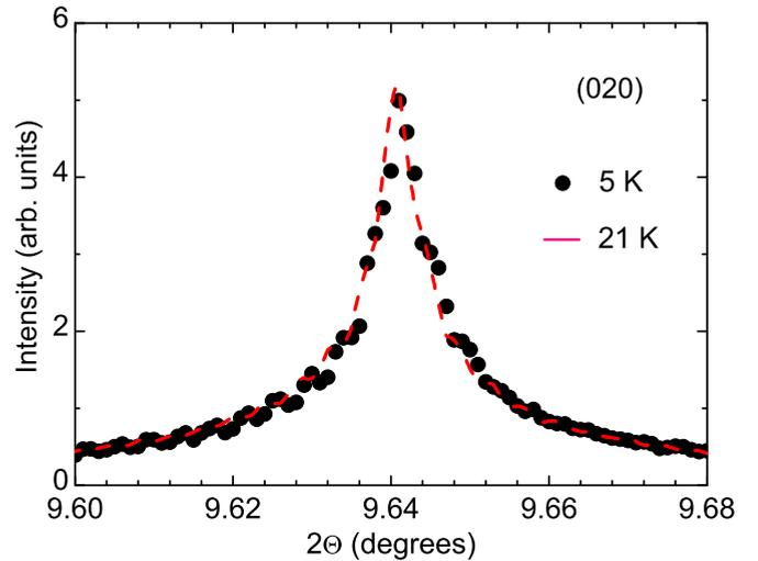
FIG. 2. The (020) Bragg peak measured at 5 K (black circles) and 21 K (red dashed line). Neither splitting nor broadening of the line shape is observable, indicating that the tetragonal symmetry is preserved in the superconducting phase.
