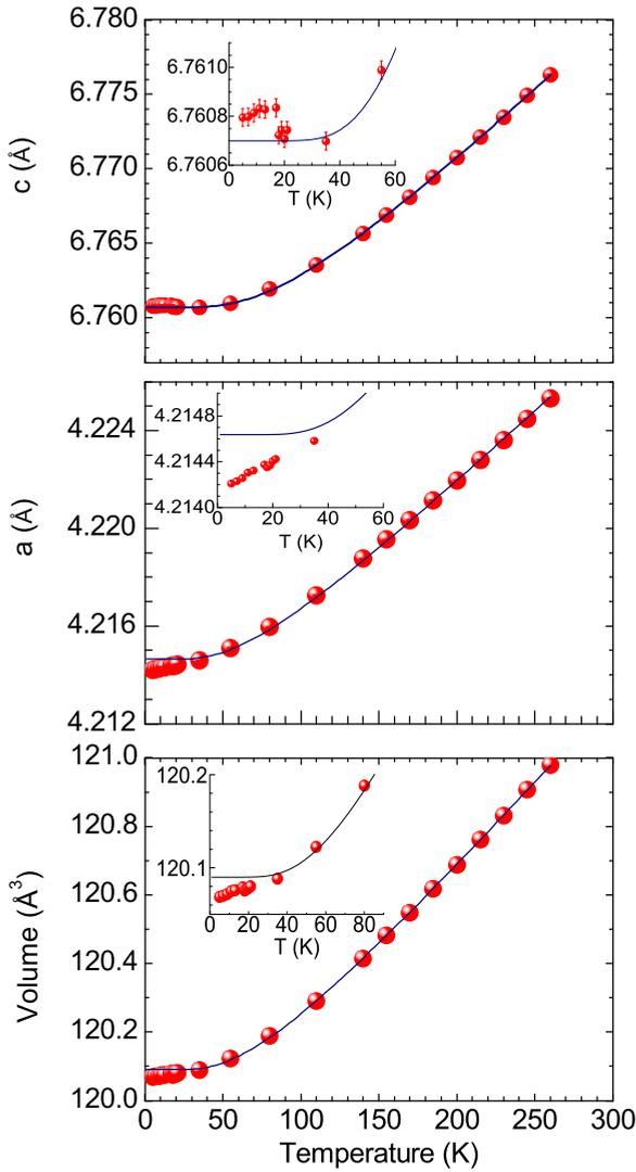
FIG. 3. Thermal expansion of the PuCoGa<sub>5</sub> lattice parameters and unit-cell volume. The solid lines represent a fit to a Grüneisen-Einstein model as explained in the text. The vertical bars give the statistical error multiplied by a factor of 5. If not visible, the error bars are smaller than the symbol sizes.
