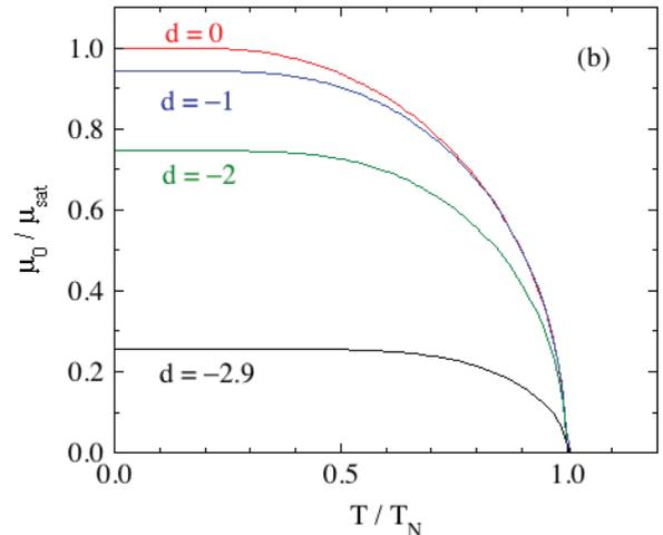
FIG. 30. Reduced ordered moment  $\bar{\mu}_0 = \mu_0/\mu_{\text{sat}}$  versus reduced temperatures (a)  $T/T_{NJ}$  and (b)  $T/T_N$  calculated using Eqs. (143) for spins  $S = 1$  with  $x$ -axis collinear AFM ordering with reduced anisotropy parameters  $d = D/k_B T_{NJ} = 0, -1, -2$ , and  $-2.9$ .
