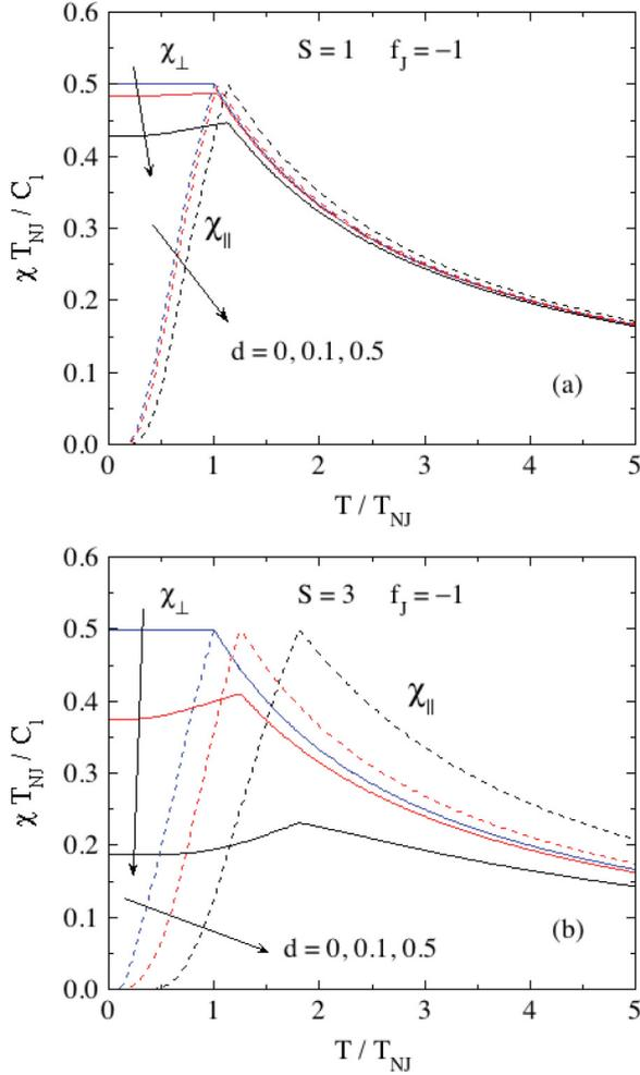
FIG. 24. Normalized magnetic susceptibilities  $\bar{\chi} \equiv \chi T_{NJ}/C_1$  where  $\bar{\chi} = \bar{\chi}_{\perp}$  (solid curves) and  $\bar{\chi} = \bar{\chi}_{\parallel}$  (dashed curves) versus  $t = T/T_{NJ}$  obtained using Eqs. (119) and (90a), respectively, with  $f_J = -1$  and  $d = 0, 0.1, \text{ and } 0.5$  for spins (a)  $S = 1$  and (b)  $S = 3$ .
