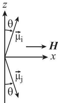
FIG. 22. Geometry of two representative ordered moments  $\vec{\mu}_i$  and  $\vec{\mu}_j$  in the AFM phase with a field applied along the perpendicular  $x$  axis. Both moments have equal magnitudes and make equal angles  $\theta$  with respect to the easy  $z$  axis.
