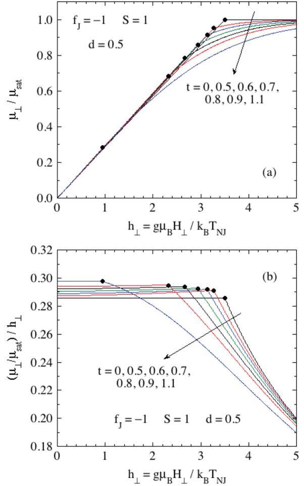
FIG. 26. (a) Reduced magnetization  $\bar{\mu}_{\perp} = \mu_{\perp}/\mu_{\text{sat}}$  versus reduced field  $h_{\perp}$  for the listed values of reduced temperature  $t$  for  $f_J = -1$ ,  $d = 0.5$ , and  $S = 1$ . (b) Ratio of  $\bar{\mu}_{\perp}/h_{\perp}$  versus  $h_{\perp}$  for the same temperatures as in (a). The filled black circles in (a) and (b) denote the normalized perpendicular critical fields  $h_{c\perp}$ .
