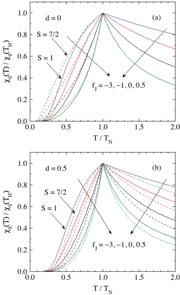
FIG. 10. Normalized parallel susceptibility  $\chi_{||}(T)/\chi_{||}(T_N)$  versus  $T/T_N$  obtained using Eq. (90b) for the listed values of  $f_J$  and spins  $S = 1$  (solid curves) and  $S = 7/2$  (dashed curves) for (a)  $d = 0$  and (b)  $d = 0.5$ .
