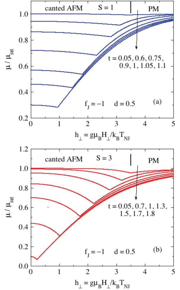
FIG. 29. Dependence of the magnitude  $\bar{\mu}$  on the reduced perpendicular field  $h_{\perp}$  at the listed temperatures for spins (a)  $S = 1$  and (b)  $S = 3$ . The cusps in the data occur at the transition field between the canted AFM state at the lower fields and the PM state at higher fields, as indicated for  $t = 0.05$  in each panel.
