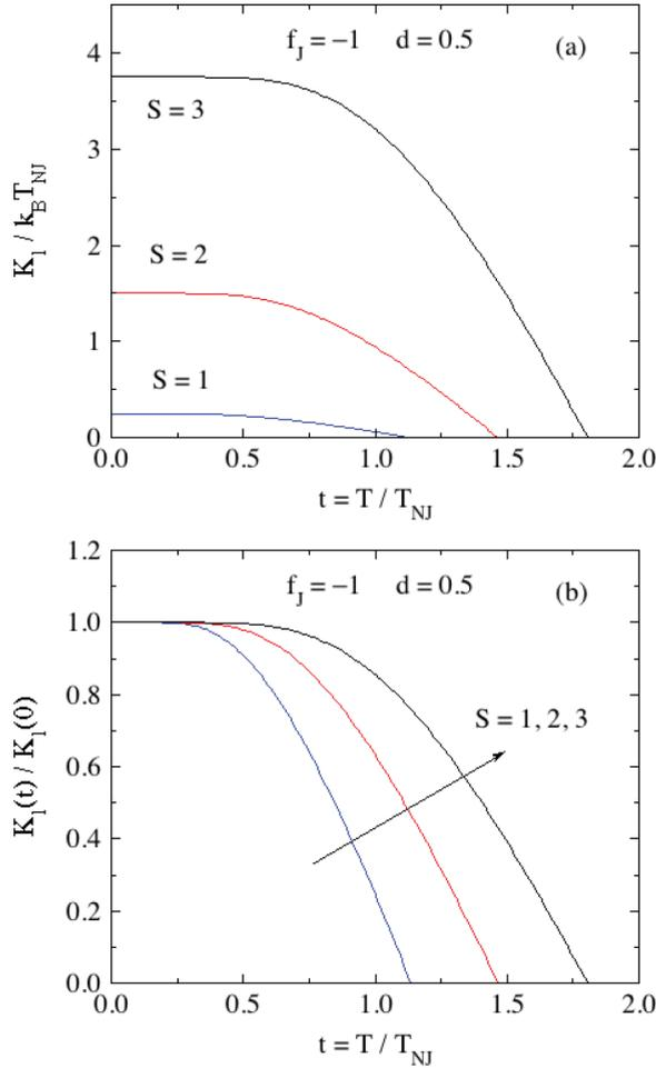
FIG. 25. Normalized anisotropy constant (a)  $K_{\perp}(t)/k_B T_{NJ}$  and (b)  $K_{\perp}(t)/K_{\perp}(0)$  for integer spins  $S = 1, 2,$  and  $3$  and  $d = 0.5$  versus reduced temperature  $t$  obtained using Eq. (132).
