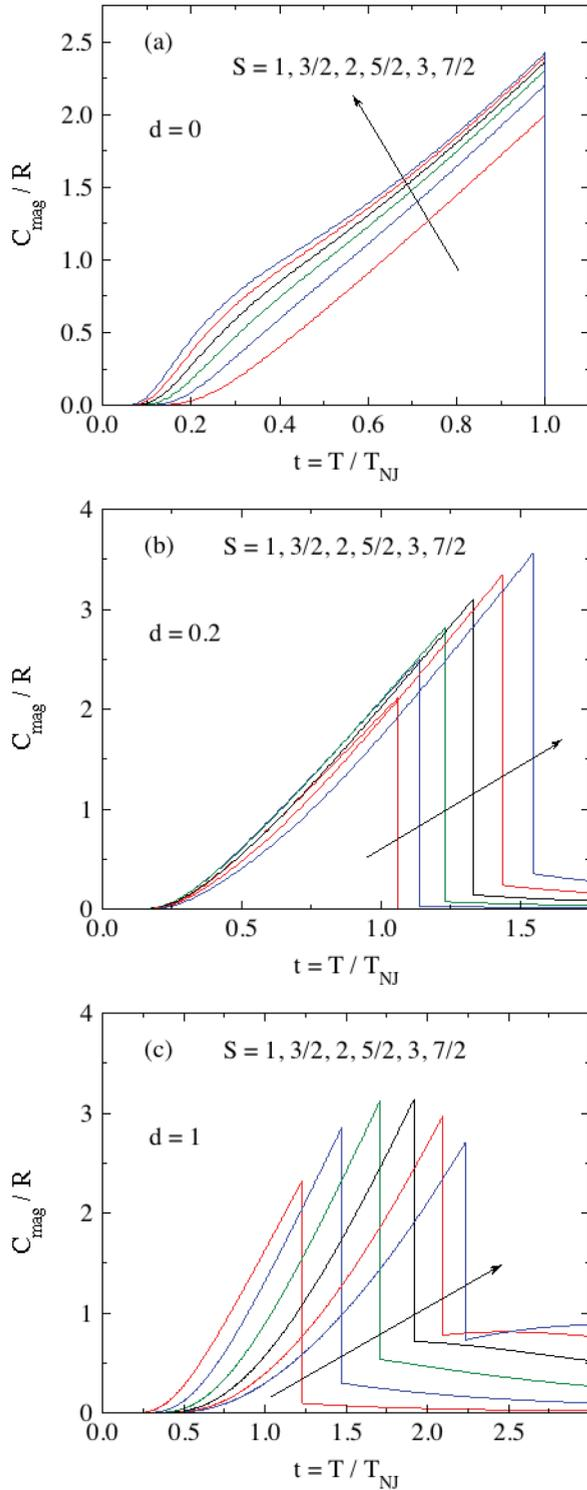
FIG. 7. Molar magnetic heat capacity  $C_{\text{mag}}/R$  versus reduced temperature  $t$  in  $H = 0$  for spins  $S = 1$  to  $7/2$  with reduced anisotropy constants  $d = D/k_B T_{\text{NJ}}$  of (a) 0, (b) 0.2, and (c) 1, calculated using Eq. (28a).
