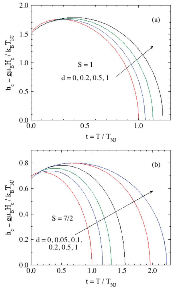
FIG. 12. Reduced  $z$ -axis critical fields  $h_c$  for  $z$ -axis collinear AFM ordering with  $f_J = -1$  versus reduced temperature  $t$  for the listed values of the anisotropy parameter  $d = D/k_B T_{NJ}$  for spins (a)  $S = 1$  and (b)  $S = 7/2$ .
