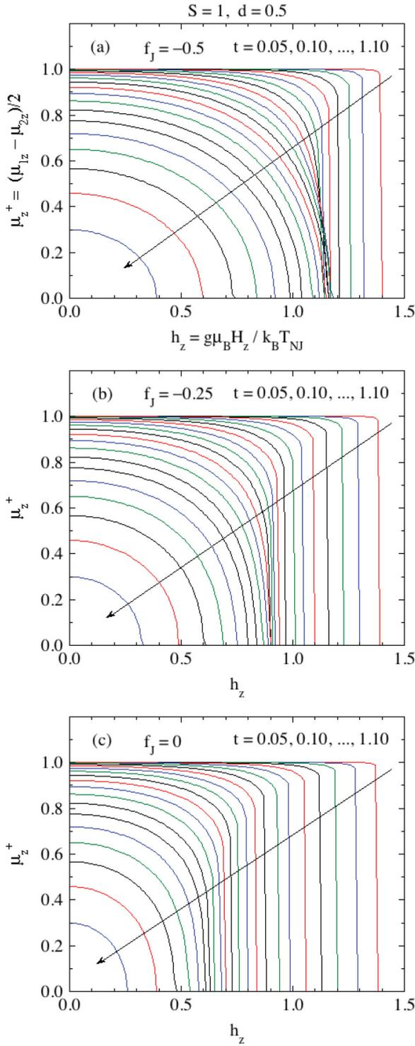
FIG. 13. Staggered  $z$ -axis moment  $\mu_z^+$  (AFM order parameter) versus reduced field  $h_z$  for the listed values of reduced temperature  $t$  for spins  $S = 1$  with reduced anisotropy parameter  $d = 0.5$  and parameter  $f_J = \theta_{PJ}/T_{NJ}$  given by (a)  $f_J = -0.5$ , (b)  $f_J = -0.25$ , and (c)  $f_J = 0$ .
