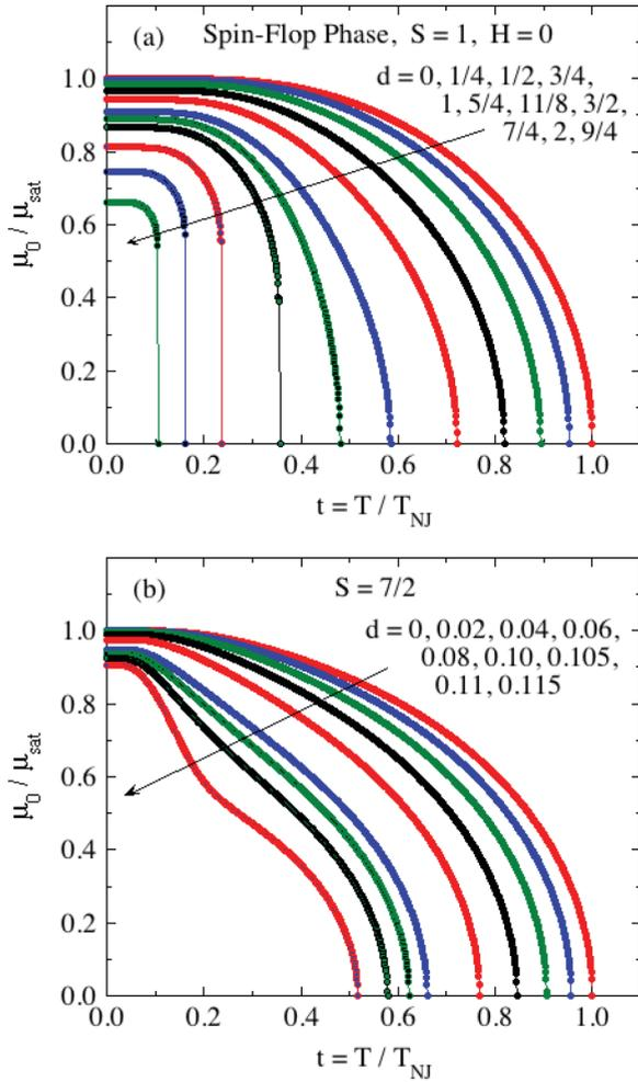
FIG. 17. Reduced ordered moment  $\bar{\mu}_0$  of the spin-flop phase in zero field for (a)  $S = 1$  and (b)  $S = 7/2$  for the listed values of reduced anisotropy parameter  $d$ , calculated from Eqs. (102). Several transitions in (a) are seen to be first order for sufficiently large  $d$ , consistent with Fig. 16. The  $d$  values for  $S = 7/2$  in (b) are small enough that all transitions shown are second order (cf. Fig. 16).
