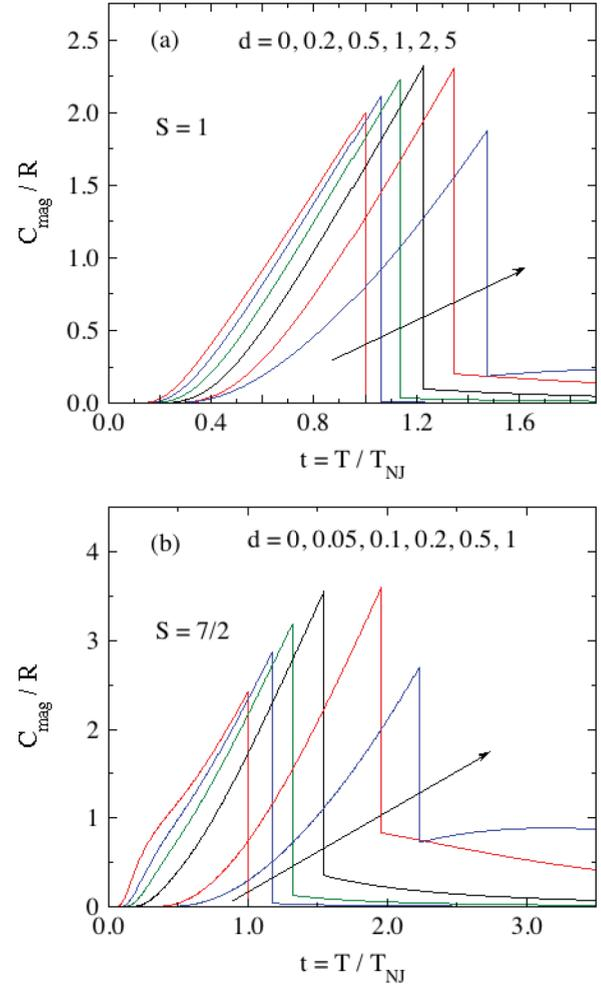
FIG. 8. Molar magnetic heat capacity  $C_{\text{mag}}/R$  versus reduced temperature  $t$  for the listed reduced anisotropy parameters  $d$  and spins (a)  $S = 1$  and (b)  $S = 7/2$ .
