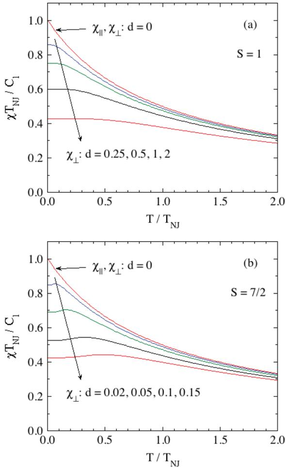
FIG. 1. Reduced parallel and perpendicular paramagnetic susceptibilities  $\bar{\chi}_{\parallel}$  with  $d = 0$  and  $\bar{\chi}_{\perp}$  for the listed values of reduced anisotropy constants  $d = D/k_B T_{NJ}$  for spins (a)  $S = 1$  obtained from Eq. (59) and (b)  $S = 7/2$  obtained from Eq. (63).
