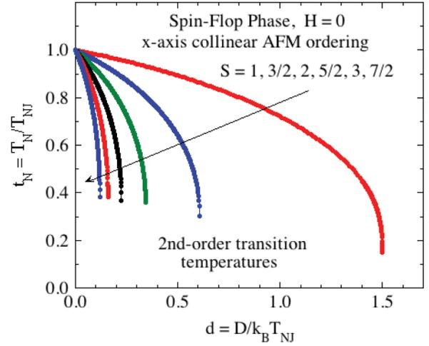
FIG. 16. Reduced transition temperature  $t_N$  of the spin-flop phase versus reduced anisotropy parameter  $d$  calculated from Eqs. (100) for the listed spin values. These data give the  $t_N$  and  $d$  ranges for second-order transitions of  $\bar{\mu}_0$  versus temperature. The missing part of each curve gives the  $t_N$  range for first-order transitions [see Fig. 17(a) for  $S = 1$  below].
