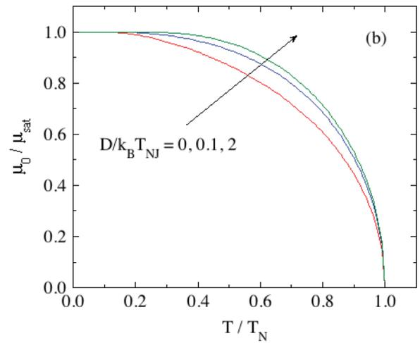
FIG. 2. Reduced ordered moment  $\bar{\mu}_0 = \mu_0/\mu_{\text{sat}}$  versus reduced temperatures (a)  $t = T/T_{NJ}$  and (b)  $T/T_N$  for z-axis collinear ordering in  $h_z = 0$  with spins  $S = 1$  and reduced anisotropy constants  $d = D/k_B T_{NJ} = 0, 1$ , and  $2$  obtained by solving Eq. (69).
