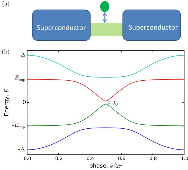
FIG. 1. (a) JJ configuration showing FAJE consists of a high transparency channel connecting two superconductors. The channel is tunnel coupled to an impurity bound state (shown as a disk adjoining wire). (b) Computed Andreev bound state spectrum for the setup in (a) shows a weakly avoided crossing at  $E = 0$  and a gap to higher-energy states generated by a larger avoided crossing with the flat impurity bound state. The weakly avoided crossing can lead to an FAJE at finite voltages.
