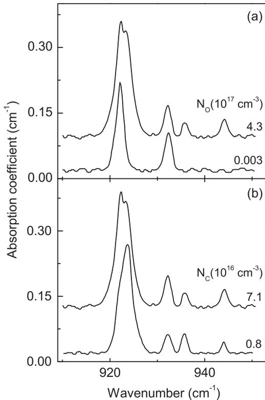
FIG. 5. Dependence of the  $923.5 \text{ cm}^{-1}$  absorption line (a) on the oxygen (samples 4 and 5) and (b) carbon (samples 4 and 6) contents in Si. The oxygen and carbon concentrations for initial samples are shown on the right. The irradiation dose was  $\Phi = 5 \times 10^{17} \text{ cm}^{-2}$ .
