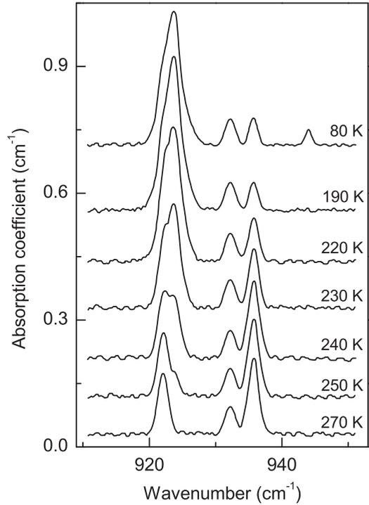
FIG. 6. Evolution of the absorption spectrum at the 20 min isochronal annealing in the temperature interval from 80 to 270 K for irradiated  $^{28}\text{Si}$  (sample 7). Irradiation dose was  $\Phi = 6 \times 10^{17} \text{ cm}^{-2}$ . The spectra are vertically shifted for clarity.
