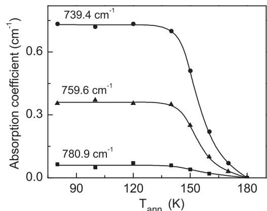
FIG. 3. Changes in the intensities of revealed absorption lines at the 20 min isochronal annealing of the irradiated boron-doped Si (sample 2). The concentration of boron in the untreated sample was  $N_B = 3.6 \times 10^{16} \text{ cm}^{-3}$ . Irradiation dose was  $\Phi = 5 \times 10^{17} \text{ cm}^{-2}$ .
