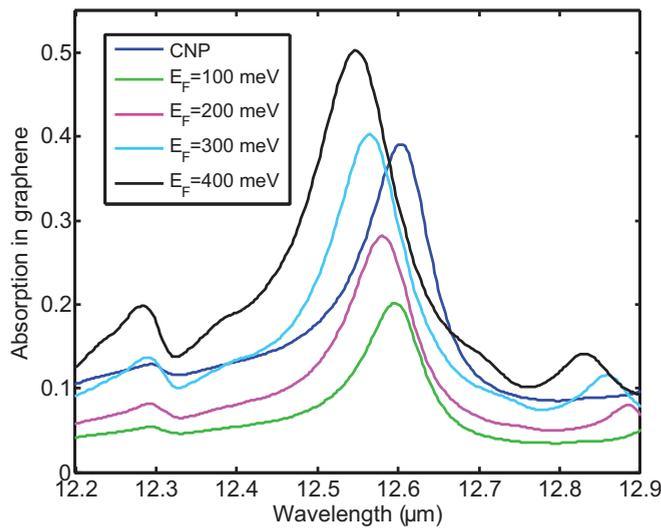
FIG. 9. The absorption by the graphene layer for the device plotted in the inset of Fig. 7.
