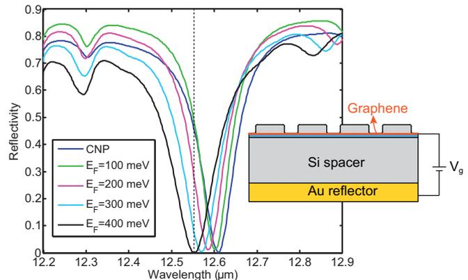
FIG. 8. The reflection spectra of the graphene-PHC optical modulator when graphene is gated to different Fermi energies. The dashed line marks the operating wavelength at  $12.55 \mu\text{m}$ .  $E_F = 100 \text{ meV}$  and  $400 \text{ meV}$  correspond to the ON and OFF state of the optical modulator, respectively. The inset shows the device structure.
