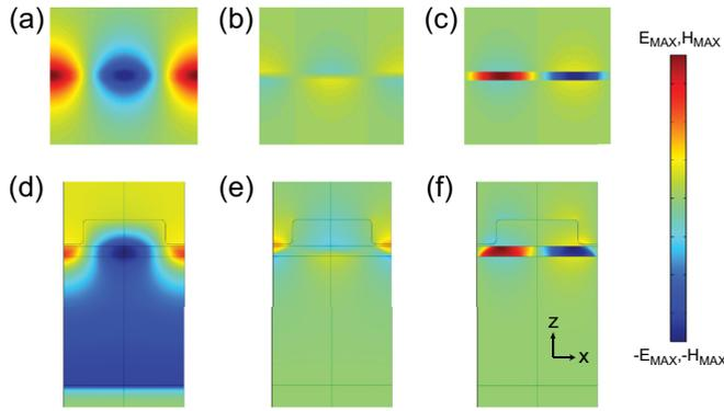
FIG. 3. (a)  $H_y$ , (b)  $E_x$ , and (c)  $E_z$  of the counter-propagating  $TM_0$  waveguide modes (backward branch) in a waveguide of 50-nm-thick h-BN slab sandwiched by amorphous silicon at the wavelength of  $12.62 \mu\text{m}$ . (d)  $H_y$ , (e)  $E_x$ , and (f)  $E_z$  of the PHC-based perfect absorber simulated using FEM at the wavelength of  $12.62 \mu\text{m}$ . The  $E_x$  and  $E_z$  are plotted with a quarter cycle time difference relative to  $H_y$ .
