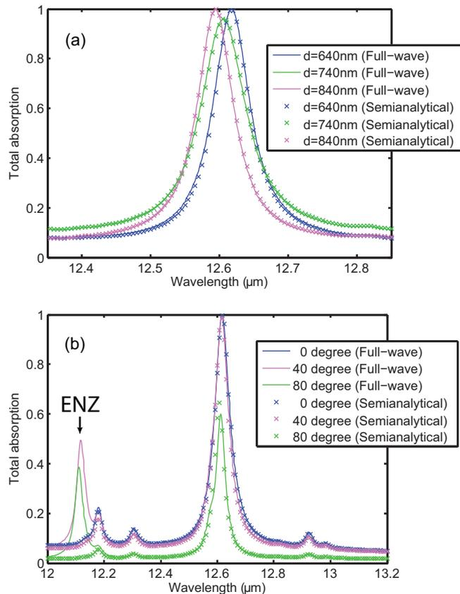
FIG. 6. (a) The absorption spectra of the PHC-based absorber with different spacer thicknesses. (b) The absorption spectra of the PHC-based absorber with different incidence angles. The results obtained from both full-wave FEM simulation and semianalytical calculation are plotted for comparison.
