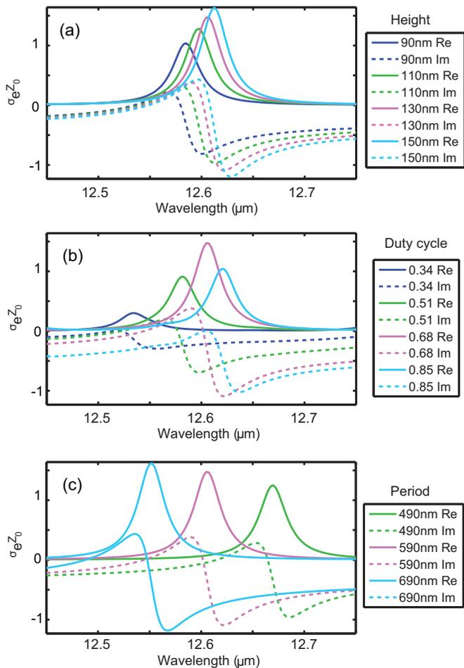
FIG. 7. The effective electric sheet conductivity  $\sigma_e$  of the PHC slab obtained with different grating heights (a), duty cycles (b), and periods (c). All other dimensions are kept the same as described in the caption of Fig. 1.
