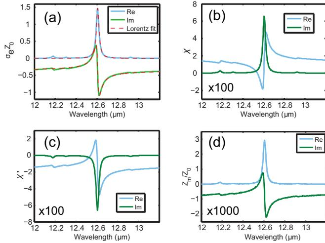
FIG. 4. Parameters for the equivalent metasurface of the PHC slab. (a)  $\sigma_e$ , (b)  $\chi$ , (c)  $\chi'$ , (d)  $Z_m$ . Notice that (b) and (c) are scaled by 100 times and (d) is scaled by 1000 times for clarity. We also perform a Lorentz fit to (a).
