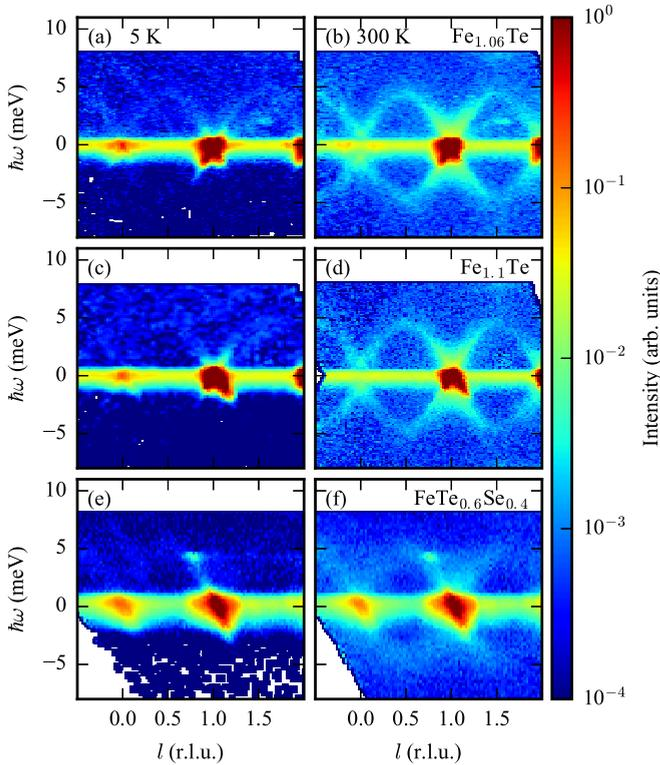
FIG. 1. Neutron scattering intensity along  $(1,0,l)$  as a function of energy transfer  $\hbar\omega$ , showing the phonon dispersions from  $(100)$ ,  $(101)$ , and  $(102)$  at 5 K (left column) and 300 K (right column) for (a)–(b)  $\text{Fe}_{1.06}\text{Te}$ , (c)–(d)  $\text{Fe}_{1.1}\text{Te}$ , and (e)–(f)  $\text{FeTe}_{0.55}\text{Se}_{0.45}$ .
