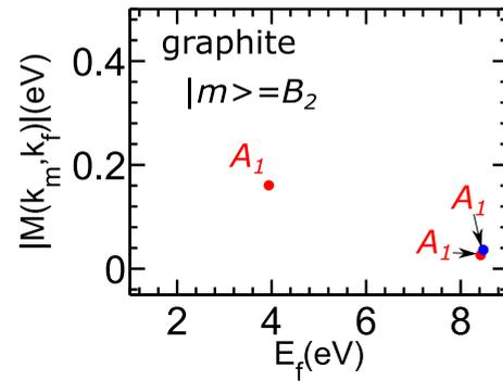
FIG. 8. Electron-phonon matrix elements for the ZA phonon mode of graphite for the transitions from an intermediate state  $|m\rangle$  having  $B_2$  symmetry (the  $\pi^*$  band near the  $K$  point) into some different final states with energies  $E_f$ .
