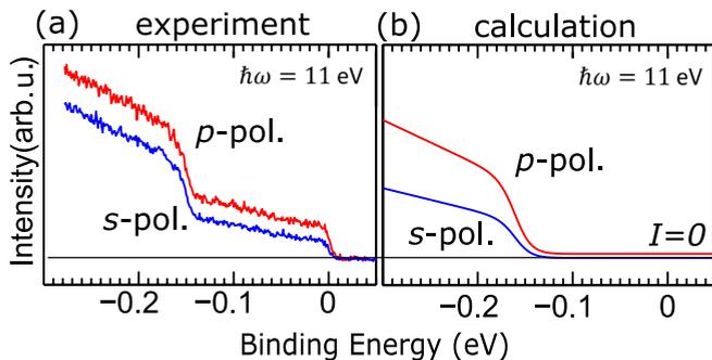
FIG. 9. (a) Experimental measurement and (b) theoretical calculation of the ARPES intensity as a function of the binding energy for a single crystal of graphite. The energy of the incident photon is  $\hbar\omega = 11$  eV. The top and bottom curves correspond to the ARPES intensity for  $s$ -polarized and  $p$ -polarized light, respectively.
