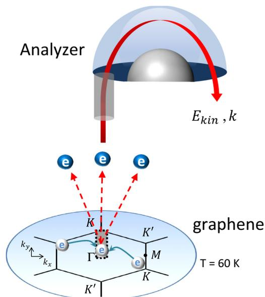
FIG. 4. The indirect scattering of an electron. An electron around the  $K$  or  $K'$  point scatters around the  $\Gamma$  point by the indirect transition. The shaded region line along  $\Gamma$ - $K$  is what we observed for  $E_{kin}$  and  $\mathbf{k}$ .
