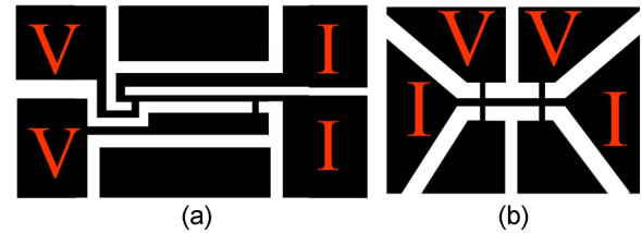
FIG. 1. Schematics of sample patterns (not to scale) and lead arrangements. Actual voltage (V) and current (I) contacts are far removed ( >1 mm) from the bridges. (a) Four-probe bridge with a folded current path. (b) Four-probe bridge with a straight through current path and voltage contacts on one side.
