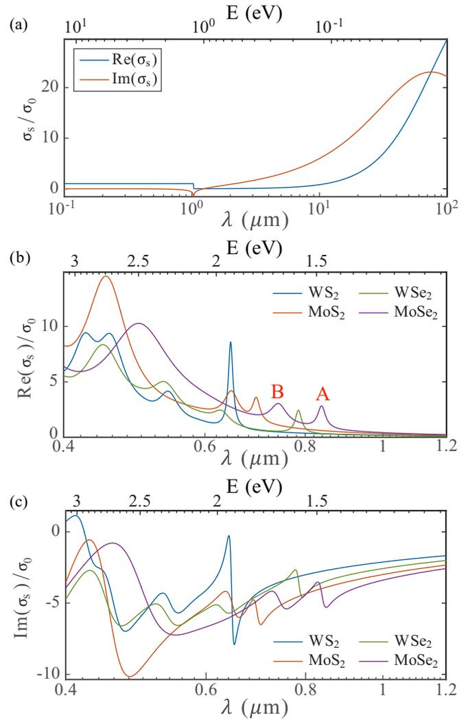
FIG. 2. (a) Dispersion of the complex sheet conductance  $\sigma_s(\omega)$  of graphene in interband and intraband wavelength range. (b), (c) Frequency dependence of the real and imaginary parts of the sheet conductance of several TMDC monolayer materials, respectively.
