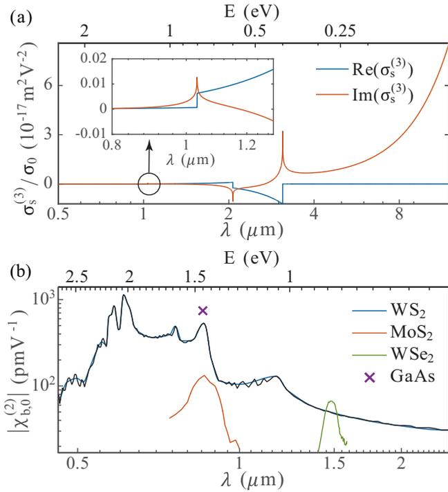
FIG. 4. (a) Real and imaginary parts of the third-order nonlinear surface conductivity of graphene  $\sigma_s^{(3)}$ . (b) Spectral dependence of the effective bulk quadratic nonlinear susceptibility  $|\chi_{b,0}^{(2)}|$  of three TMDC monolayer materials and the value of the dominant component of  $\chi_{b,xyz}^{(2)}$  for GaAs, given for reference. For WS<sub>2</sub>, the experimental noisy data (black line) has been smoothed out (blue line).
