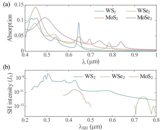
FIG. 15. (a) The FF absorption spectra for ribbons made of WS<sub>2</sub>, MoS<sub>2</sub>, WSe<sub>2</sub>, and MoSe<sub>2</sub>. (b) The SH radiation spectra for ribbons made of WS<sub>2</sub>, MoS<sub>2</sub>, and WSe<sub>2</sub>.
