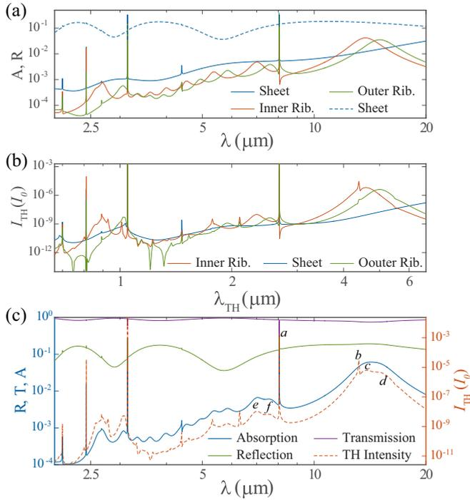
FIG. 19. (a) Absorption spectra (solid lines) of the homogeneous graphene sheet and the graphene ribbons on top of inner and outer parts of the slab waveguide [cf. Figs. 16(a)–16(c)] and reflection spectrum (dashed line) of the homogeneous graphene sheet. (b) The nonlinear radiation spectrum of the same structures as in (a). (c) Linear spectra (reflection, transmission, and absorption) and TH spectrum for the graphene ribbons placed on top of both parts of the waveguide, as per Fig. 16(d).
