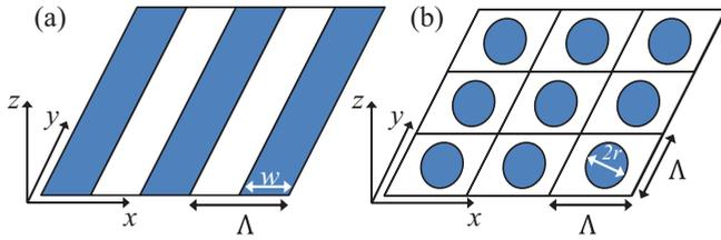
FIG. 7. Generic structures for numerical convergence analysis. (a) 1D periodic array of graphene ribbons with period  $\Lambda$  and width  $w$ . (b) 2D array of circular graphene disks with radius  $r$  and periods  $\Lambda_1 = \Lambda_2 = \Lambda$ .
