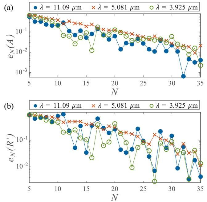
FIG. 13. (a), (b) Relative self-error for linear absorption and intensity of TH radiation, respectively, determined at the plasmon resonance wavelengths  $\lambda = 11.09 \mu\text{m}$  (dots),  $5.081 \mu\text{m}$  (crosses), and  $3.925 \mu\text{m}$  (circles).
