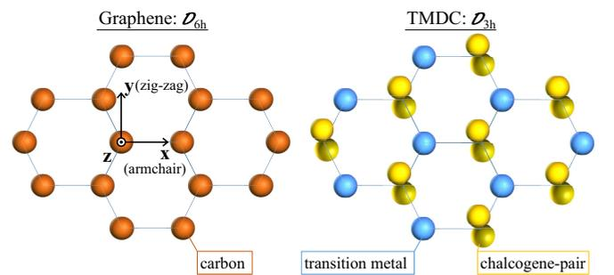
FIG. 3. Schematic of the atomic structures of graphene (symmetry group  $\mathcal{D}_{6h}$ , left) and TMDC monolayers (symmetry group  $\mathcal{D}_{3h}$ , right). The hexagonal lattice of graphene is centrosymmetric and thus SHG is forbidden. By contrast, the lattice of TMDC monolayers is noncentrosymmetric and as such SHG is allowed.
