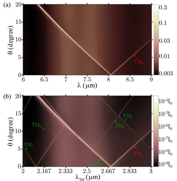
FIG. 21. (a) Map of absorption spectra vs angles of incidence  $\theta$  determined in the wavelength range of the second-order surface plasmon of graphene ribbons. (b) The map of nonlinear radiation spectra shows the inherited (red labels) and intrinsic, nonlinear (green labels) modes of the slab waveguide. The left and right branches of intrinsic modes of the same order exhibit anticrossing mode interaction, which leads to the formation of spectral band gaps.
