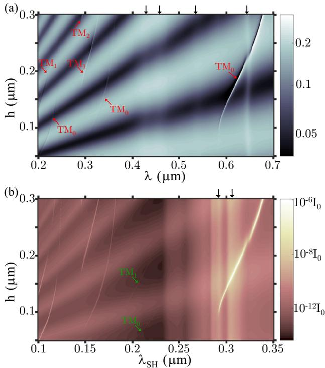
FIG. 18. (a) Map of linear reflection spectra vs waveguide height  $h$  exhibits Fabry-Perot resonances, resonances due to exciton generation ( $\downarrow$ ) and resonances due to excitation of waveguide modes ( $\searrow$ ). Interaction between the  $\text{TM}_0$  waveguide mode and excitons of  $\text{WS}_2$  monolayer as well as Fano resonances can be observed. (b) Map of nonlinear radiation spectra determined for different waveguide height  $h$ .
