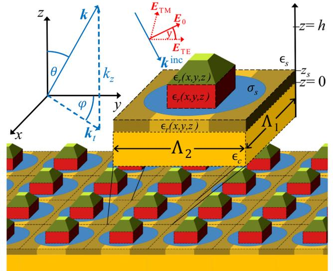
FIG. 1. Schematic of a generic multilayer structure periodic along the  $x$  and  $y$  directions under plane-wave incidence, and a closeup of the unit cell. The distribution of the 2D material (blue) is defined by the position-dependent sheet conductance  $\sigma_s(x, y, z_s)$  at  $z = z_s$ . The bulk part of the periodic structure, which can consist of slanted (olive green), straight walled (red), or embedded parts (sand brown), is defined by the permittivity function  $\epsilon_r(x, y, z)$ .
