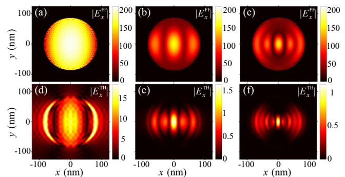
FIG. 14. Dominant electric field component  $|E_x|$  at the FF (top panels) and TH (bottom panels) at the surface of a graphene disk for the resonance wavelengths, from left to right,  $\lambda_{\text{FF}} = 11.09, 5.081$ , and  $3.925 \mu\text{m}$ . The number of harmonics used in the simulations was  $N = 40$  at the FF and  $N = 30$  at the TH.
