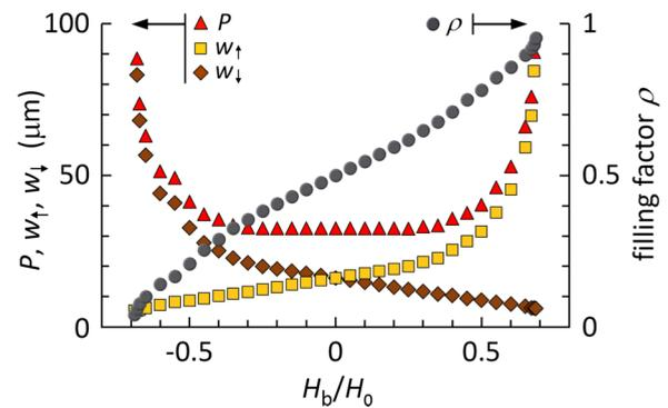
FIG. 2. Normalized field dependences of the domain structure period  $P$  (triangles), the oppositely magnetized domain widths  $w_{\uparrow}$  (squares) and  $w_{\downarrow}$  (diamonds), and the domain structure filling factor  $\rho$  (circles) of the sample. The bias field  $H_b$  is directed along the normal to the sample surface and normalized to the bubble collapse field  $H_0$ .
