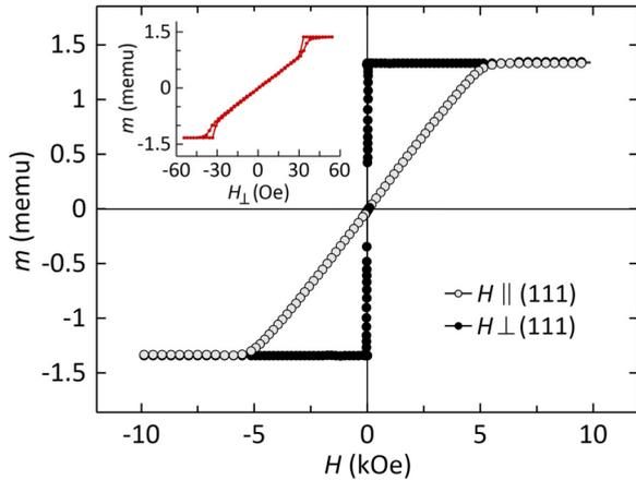
FIG. 3. Magnetic hysteresis loops  $m(H)$  of the garnet film for two directions of the magnetic field: parallel ( $H_{\parallel}$ , gray circles) and perpendicular ( $H_{\perp}$ , black circles) to the film plane. Inset: the magnetic hysteresis loop  $m(H_{\perp})$  when the field  $H_{\perp}$  varies in a range of  $\pm 100$  Oe.
