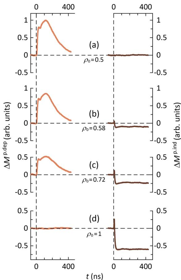
FIG. 6. Time evolution of the sample's magnetization normal component change corresponding to the contributions to the photomagnetization from the polarization-dependent [ $\Delta M^{p.dep}(\rho_0, t)$ , left] and the polarization-independent [ $\Delta M^{p.ind}(\rho_0, t)$ , right] effects after the mathematical processing of the photomagnetization pulses  $\Delta M(\rho_0, t)$  (Fig. 5).
