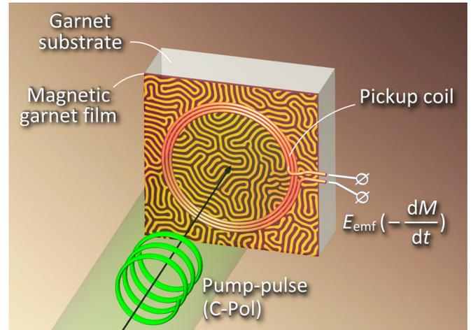
FIG. 1. Scheme of the experiment for the pulsed photomagnetization: the garnet film with a labyrinthine domain structure, a circularly polarized (C-Pol) laser pump pulse, and an inductive transducer (a pickup coil).
