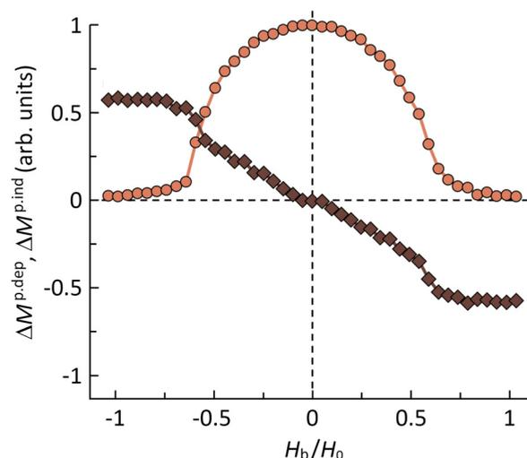
FIG. 7. Normalized field dependences of the photomagnetization pulses amplitudes  $\Delta M^{p.dep}(\rho_0, t)$  and  $\Delta M^{p.ind}(\rho_0, t)$  caused by the polarization-dependent (circles) and the polarization-independent (diamonds) effects, respectively. The bias field  $H_b$  is normalized to the bubble collapse field  $H_0$ .
