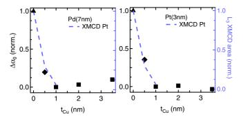
FIG. 5. Damping enhancement  $\Delta\alpha_0$  (left axis, normalized as  $\Delta\alpha_0(t_{\text{Cu}}) \rightarrow [\Delta\alpha_0(t_{\text{Cu}}) - \Delta\alpha_0(1\,\text{nm})]/[\Delta\alpha_0(0\,\text{nm}) - \Delta\alpha_0(1\,\text{nm})]$ ), due to spin pumping, as a function of interlayer thickness  $t_{\text{Cu}}$  for Py(5 nm)/Cu( $t_{\text{Cu}}$ )/N heterostructures, with N = Pd(7 nm), N = Pt(3 nm). The dashed line represents the XMCD signal (right axis) reported from inset in Fig. 2.
