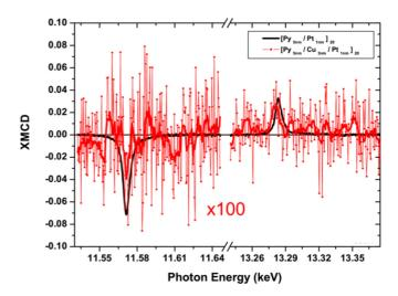
FIG. 7. X-ray absorption magnetic circular dichroism (XMCD) spectra at  $L_{3,2}$  absorption edges of Pt for  $[Py(5 \text{ nm})/Pt(1 \text{ nm})]_{20}$  (black solid line) and  $[Py(5 \text{ nm})/Cu(3 \text{ nm})/Pt(1 \text{ nm})]_{20}$  (red markers; enhanced by a factor 100) multilayers.
