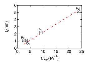
FIG. 6. Effect of direct exchange strength on length scale of spin current absorption. Cutoff thickness  $t_c$  extracted from the  $\Delta\alpha(t_N)$  data in Fig. 3 as a function of reciprocal interfacial exchange energy  $1/J_{ex}$  extracted from XMCD in Fig. 1. Labels are given in terms of  $J_{ex}$ . The Co and Py points are from Ref. [14].
