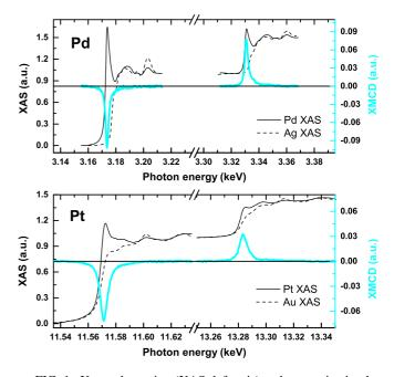
FIG. 1. X-ray absorption (XAS, left axis) and magnetic circular dichroism (XMCD, right axis) spectra at the L edges of Pd (top panel) and Pt (bottom panel) for [Py(5 nm)/Pt(1 nm)]<sub>20</sub> and [Py(5 nm)/Pd(2.5 nm)]<sub>20</sub> multilayers. The dashed traces represent XAS spectra at L edge of Ag and Au used as background of Pd and Pt, respectively, to extract the values of induced magnetic moment reported in Table I.
