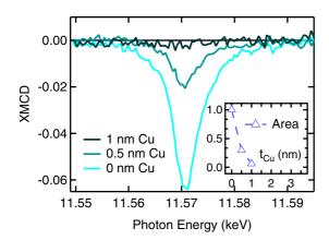
FIG. 2. XMCD spectra at the  $L_3$  edge of Pt for  $[Py(5 \text{ nm})/Cu(t_{Cu})/Pt(1 \text{ nm})]_{15}$ , with  $t_{Cu}=0$ , 0.5, and 1 nm. Inset: The area of the  $L_3$  XMCD peak is plotted as a function of Cu thickness.
