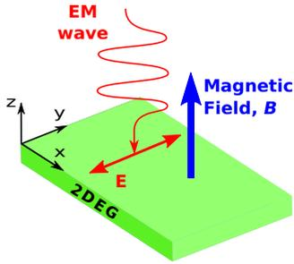
FIG. 1. Sketch of the system under consideration: Two-dimensional electron gas (2DEG) subjected to both a linearly polarized electromagnetic wave (EM) with the electric field amplitude,  $E$ , and a stationary magnetic field,  $\mathbf{B}$ , directed perpendicularly to the 2DEG plane.
