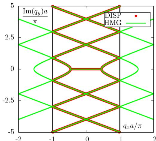
FIG. 11. An expanded view of  $\text{Im}(q_y)$  as a function of  $q_x$  for  $ka/\pi = 0.200$  [case (a)]. Here several “reflected” segments of the isofrequency line are shown. These segments are obtained by folding the corresponding isofrequency line for an infinite homogeneous medium into the FBZ of the triangular lattice according to (27). The analytical lines outside the FBZ (shown by the two vertical lines) are not the actual solutions and are shown only to guide the eye.
