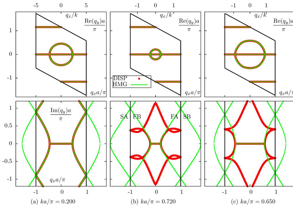
FIG. 10. Same as in Fig. 4 but for the triangular lattice of hollow cylinders. The “HMG” isofrequency lines were computed according to (22) with  $q^2 = n_{\text{eff}}^2 k^2$  and  $n_{\text{eff}}^2 = 5.20$  (a),  $n_{\text{eff}}^2 = 0.085$  (b), and  $n_{\text{eff}}^2 = 0.82$  (c). In the top row of plots, the FBZ of the lattice is shown by the black rhombus. In the lower plot (b), FA and FB mark the first pair of hyperbolas defined by (27), and SA, SB mark the second pair of hyperbolas.
