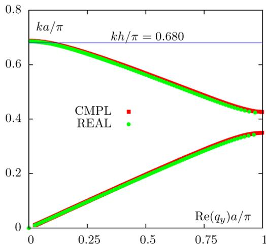
FIG. 7. Comparison of dispersion diagrams for the host material with a constant real permittivity  $\epsilon_h = 9.61$  (REAL) and with dispersive and complex permittivity given by (23) (CMPL). Geometrical parameters are the same as in Fig. 3. The horizontal line marks the frequency at which the isofrequency line has been computed for both cases. In the case of dispersive media,  $q_y$  is complex and the quantity shown on the horizontal axis is  $\text{Re}(q_y)$ .
