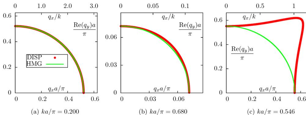
FIG. 5. Purely real parts of the isofrequency lines shown in Fig. 4. The lines marked “HMG” are ideal circles.
