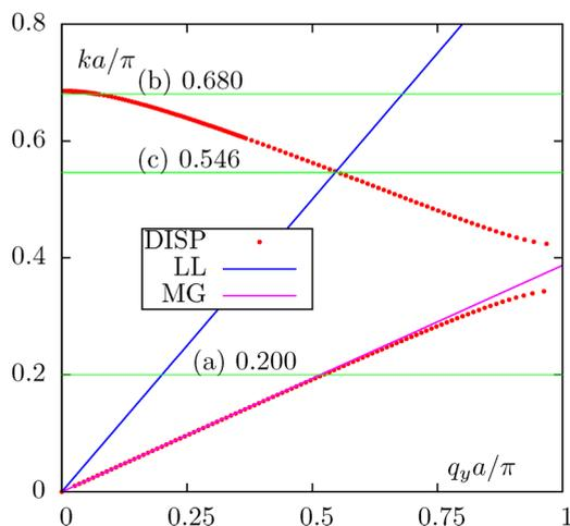
FIG. 3. Dispersion diagram for the square lattice of hollow cylinders. Frequency is scanned from zero to slightly above the second  $\Gamma$ -point frequency. The variable  $ka/\pi = \omega a/\pi c = 2a/\lambda$  is the dimensionless frequency. The line labeled LL is the light line and the line labeled MG gives the Maxwell Garnett approximation to the dispersion curve. Thin horizontal lines mark the frequencies at which further simulations have been performed.
