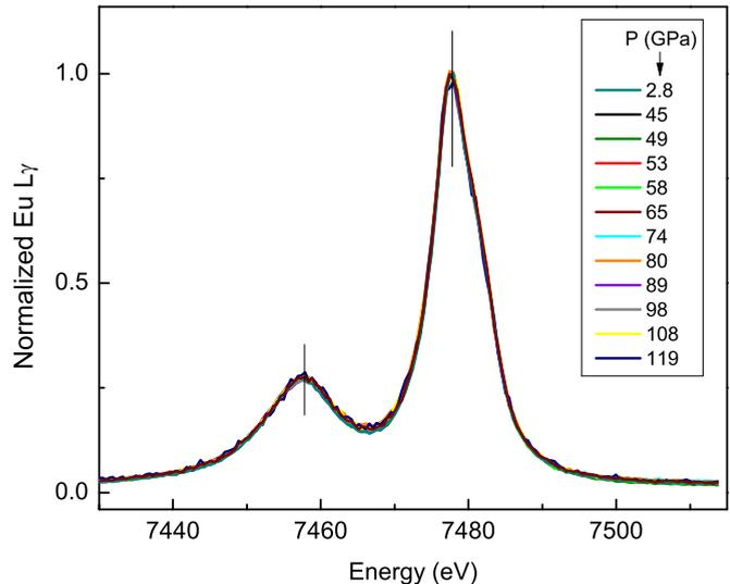
FIG. 4.  $L_{\gamma_1}$  XES spectra of Eu to pressures of 119 GPa at room temperature, normalized to main peak intensity. Vertical lines show peak positions for main band and satellite peaks. No apparent change in XES spectra was observed under pressure, suggesting no change in  $4f$  magnetic moment to 119 GPa.
