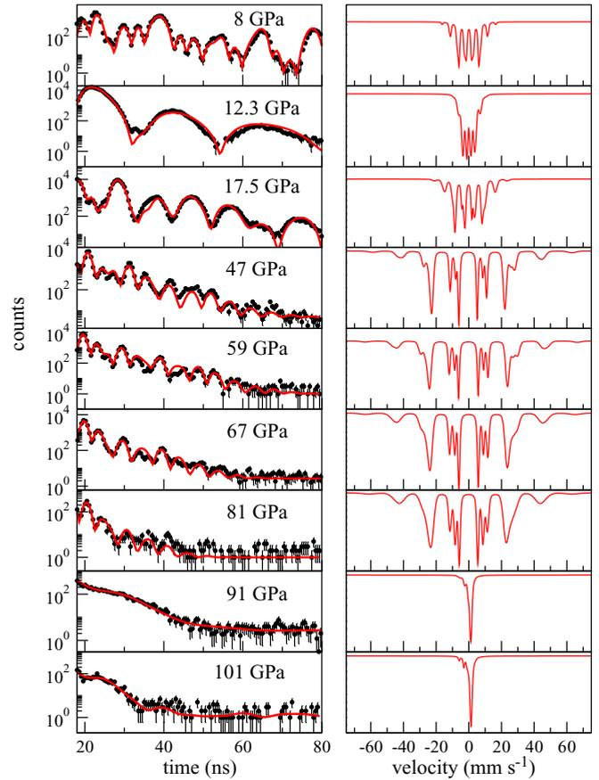
FIG. 1. (left column) Representative SMS spectra of Eu at high pressure and 11 K. Black dots are data, and red lines are fits from CONUSS. (right column) Simulated spectra in energy domain from fits of the time-domain data (red lines in left column).
