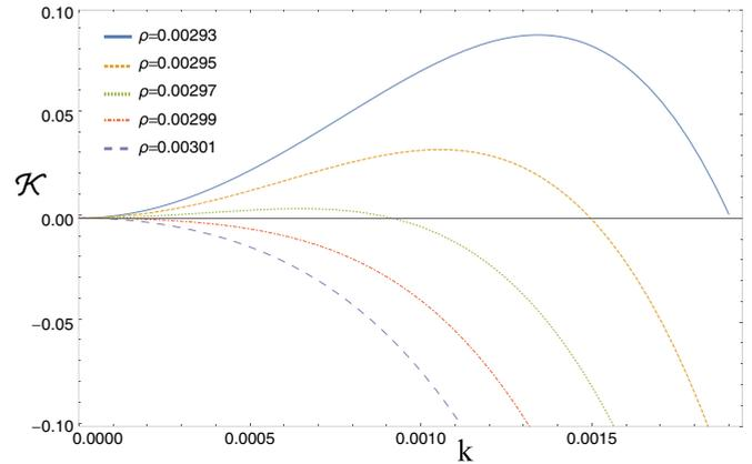
FIG. 3. The function  $\mathcal{K}(k)$  that defines the parameter  $k$  of nonuniformity of superconducting state in a single helix AF for different transition temperatures  $\rho = T/vq$  at  $\gamma = 0.1$ . The formation of  $k \neq 0$  peak as  $\rho$  decreases below  $\rho^* = 0.00297$  signals the nonuniform state below the second-order phase transition from the normal state to the superconducting state.
