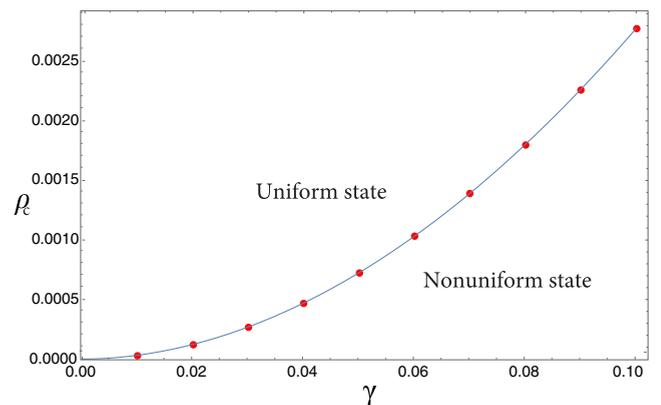
FIG. 4. The critical dimensionless temperature  $\rho_c^* = T_c/vq$ , separating transitions to the uniform and the nonuniform states, as a function of the parameter  $\gamma$  in a single helix antiferromagnet. The fit for  $\rho_c^*(\gamma)$  is  $\rho_c^* \approx 0.26\gamma^2$ .
