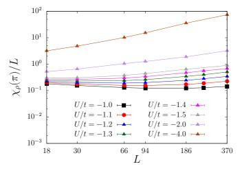
FIG. 18. (Color online) Finite-size scaling of the charge susceptibility for the U-V model. Here,  $\beta t = 2L$ , V/t = 0.1. Results obtained in the SSE representation.
