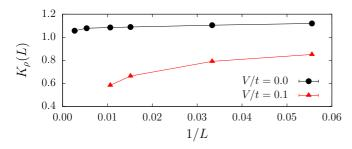
FIG. 17. (Color online)  $K_{\rho}(L)$  for the *U-V* model. Here,  $\beta t = 2L$ , U/t = -4. Results obtained in the SSE representation.
