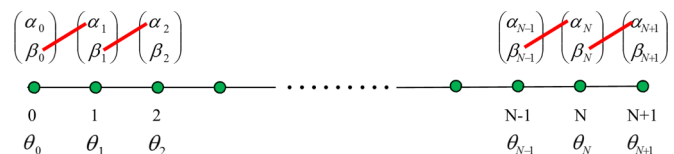
FIG. 1. (Color online) Set-up of our finite-chain QW with disorder, with totally N + 2 sites, where site 0 and N + 1 are the boundary sites with reflection operators R_- and R_+ . Rotation operators of bulk sites with n = 1, 2 \dots N - 1, N depend on the local angle \theta_n , which fluctuate from site to site. The red slashes connect spin components \beta_n and \alpha_{n+1} , as they form the new “spinor” in our transfer matrix formalism elaborated in our main text.
