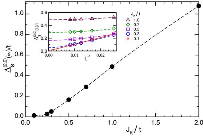
FIG. 3. (Color online) Extrapolated spin gap  $\Delta_s^{(2,0)}(\infty)$  (corresponding to the Haldane gap), as a function of  $J_K$ , obtained after a finite-size scaling analysis (see inset). Dashed lines are a guide to the eye. Inset: Finite-size scaling using the scaling law  $\Delta_s(L) \approx \sqrt{\Delta_s^2(\infty) + \beta_s L^{-2}}$ .
