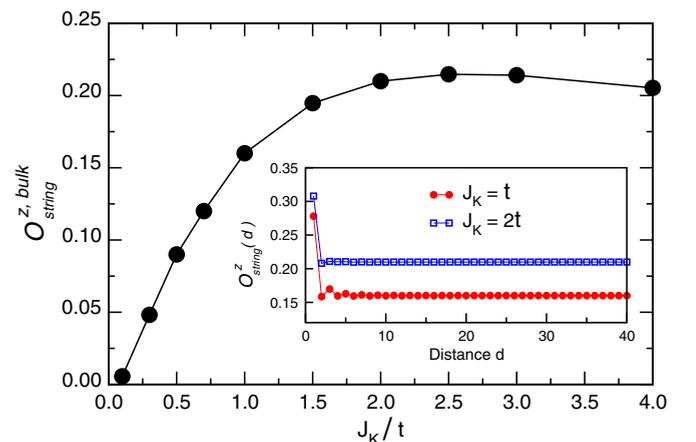
FIG. 5. (Color online) String order parameter  $\mathcal{O}_{\text{string}}^{z,\text{bulk}}$  vs  $J_K$ . Throughout the whole studied regime,  $\mathcal{O}_{\text{string}}^{z,\text{bulk}}$  remains finite, indicating the presence of a Haldane-insulating phase. Inset: Spatial dependence of  $\mathcal{O}_{\text{string}}^z(d)$  vs the distance  $d = |l-m|$ , where  $l$  and  $m$  have been taken symmetrically about the center of the chain.
