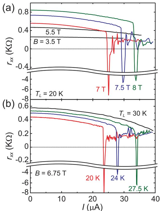
FIG. 4. (Color online) (a) Longitudinal differential resistivity  $r_{xx}$  vs  $I$  for various  $B$  at  $T_L = 20$  K. (b) Longitudinal differential resistivity  $r_{xx}$  vs  $I$  for various  $T_L$  at  $B = 6.75$  T.
