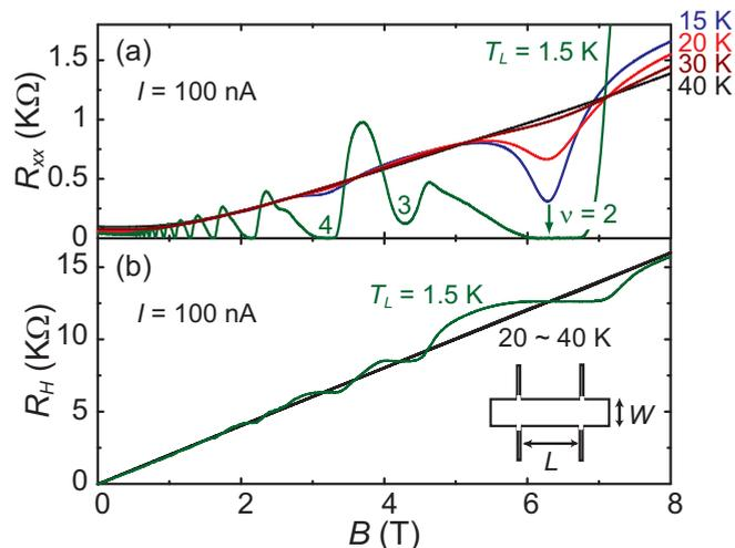
FIG. 1. (Color online) (a) Magnetic field dependence of longitudinal resistance  $R_{xx}$  for various lattice temperatures  $T_L$  and  $I = 100$  nA. (b) Magnetic field dependence of Hall resistance  $R_H$  for various lattice temperatures  $T_L$  and  $I = 100$  nA. The quantum Hall plateaus are thermally smeared out when  $T_L$  is higher than 20 K.  $R_H$  shows weak temperature dependence within  $T_L = 20$  to 40 K. The inset is a schematic of the device geometry.
