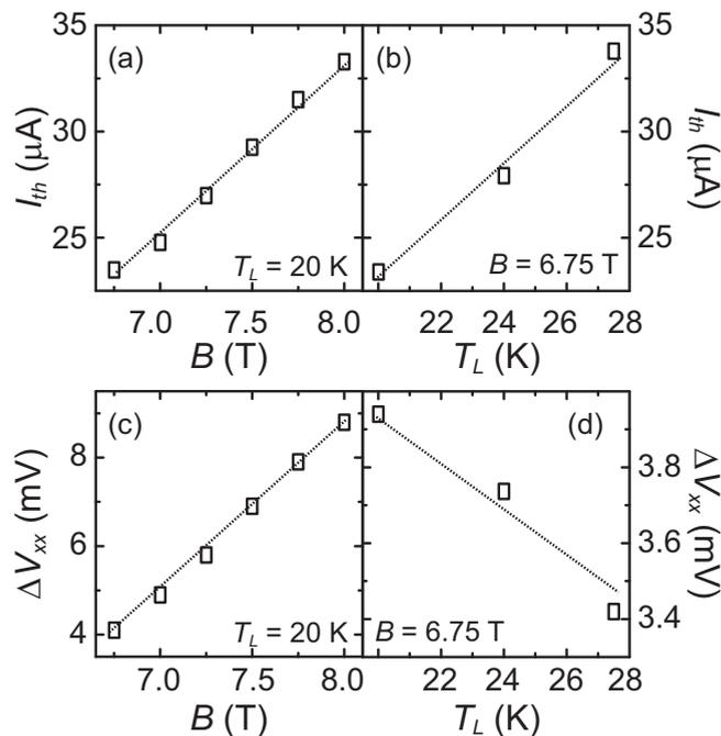
FIG. 3. Characteristics of NDR behaviors. (a)  $I_{th}$  vs  $B$  plot. (b)  $I_{th}$  vs  $T_L$  plot. (c)  $\Delta V_{xx}$  vs  $B$  plot. (d)  $\Delta V_{xx}$  vs  $T_L$  plot.
