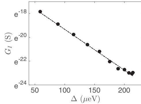
FIG. 6. Magnetic field dependence of the conductance in the injection regime for device A at  $T = 20$  mK. The conductance at  $V = 4$  mV,  $G_I$ , is plotted against the experimentally determined  $\Delta(B_{\parallel}^2)$ . The dot-dashed line is a fit to the expression  $\ln G_I = \ln G_I^0 - \Delta/k_B T_{\text{eff}}$ , which yields  $T_{\text{eff}} = 340$  mK.
