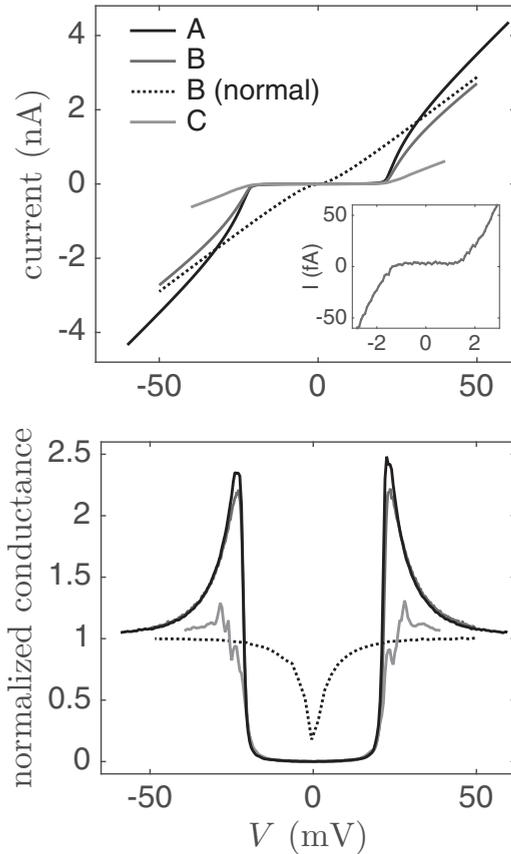
FIG. 2. (Top) Large-scale current and (bottom) conductance measurements for devices A, B, and C in the superconducting state for magnetic field  $B_{\parallel} = 0$  (solid lines) and for device B in the normal state obtained with  $B_{\parallel} = 0.7$  T (dotted lines). The inset in the top plot shows the small-scale IVC at  $T = 25$  mK for device B at femtoampere current resolution. Conductance ( $dI/dV$ ) measurements in the bottom plot are normalized to  $(NR_j)^{-1}$  for each device.
