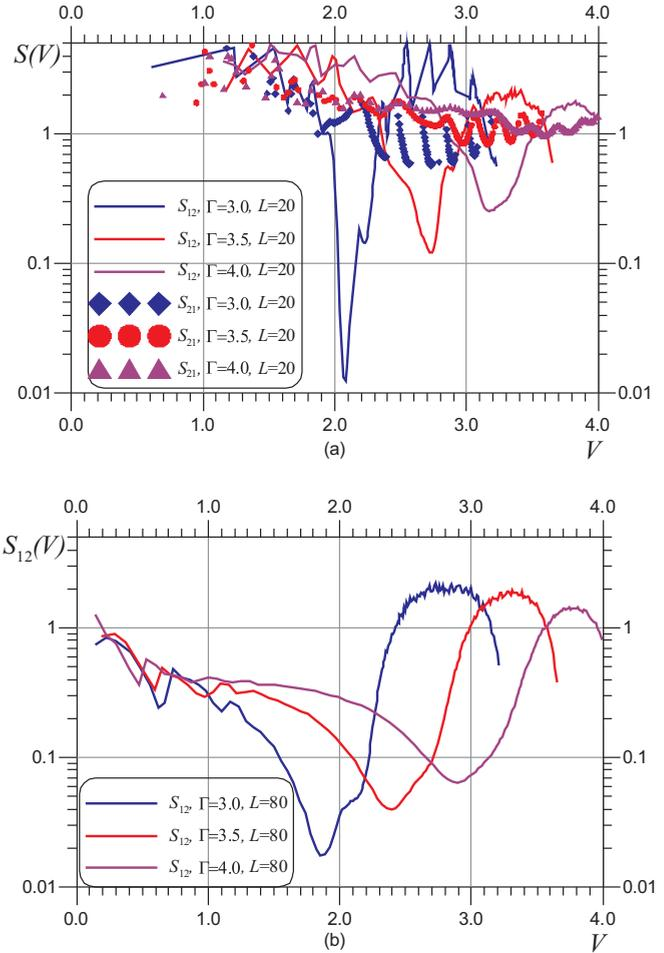
FIG. 4. (Color online) (a) The dimensionless transmitted power  $S_{12}$  and  $S_{21}$  vs dimensionless voltage for  $\alpha = 0.03$  and  $\Gamma = 3.0$ ,  $\Gamma = 3.5$ ,  $\Gamma = 4.0$ ;  $r_L = r_R = 20$ ,  $c_L = c_R = 10$ . (b) The dimensionless transmitted power  $S_{12}$  vs dimensionless voltage for  $\alpha = 0.03$  and  $\Gamma = 3.0$ ,  $\Gamma = 3.5$ ,  $\Gamma = 4.0$ ;  $r_L = r_R = 20$ ,  $c_L = c_R = 10$ ,  $L = 80$ .
