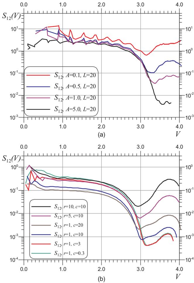
FIG. 5. (Color online) (a) The dimensionless transmitted power  $S_{12}$  vs dimensionless voltage for  $\alpha = 0.03$ ,  $L = 20$ ,  $\Gamma = 4$ ,  $r_L = r_R = 10$ , and  $c_L = c_R = 10$  for various values of driving amplitude. (b) The dimensionless transmitted power  $S_{12}$  vs dimensionless voltage for  $\alpha = 0.03$ ,  $L = 80$ ,  $A = 0.5$ , and  $\Gamma = 4$  for various values of load resistance  $r = r_L = r_R$  and capacitance  $c = c_L = c_R$ .
