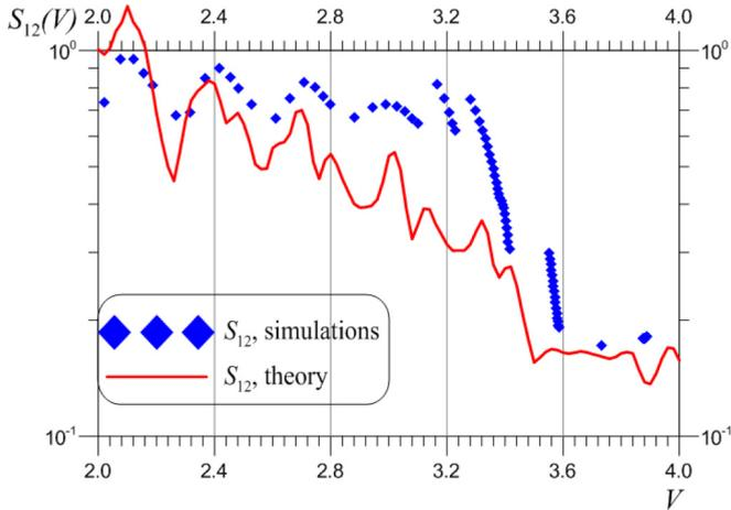
FIG. 2. (Color online) Dimensionless transmitted power  $S_{12}$  vs dimensionless voltage for  $\alpha = 0.1$ ,  $L = 20$ ,  $\Gamma = 4$ ,  $\omega = 0.231$ , and  $A = 0.5$  (the external microwave signal propagates against the flux-flow movement).
