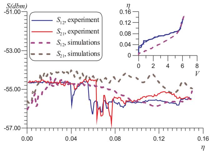
FIG. 6. (Color online) The experimentally measured dimensionless transmitted power  $S_{12}$  and  $S_{21}$  (solid curves) vs dimensionless current density compared to the numerically simulated data (dashed curves) for  $L = 18$ ,  $\alpha = 0.014$ ,  $\Gamma = 7.3$ ,  $r_L = r_R = 10$ ,  $c_L = c_R = 10$ ,  $\beta = 0.007$ ,  $\Delta\Gamma = 0.2\Gamma$ ,  $\omega = 0.231$ , and  $A = 0.5$ . The inset shows a comparison of the dimensionalized current-voltage curves for the same parameters.
