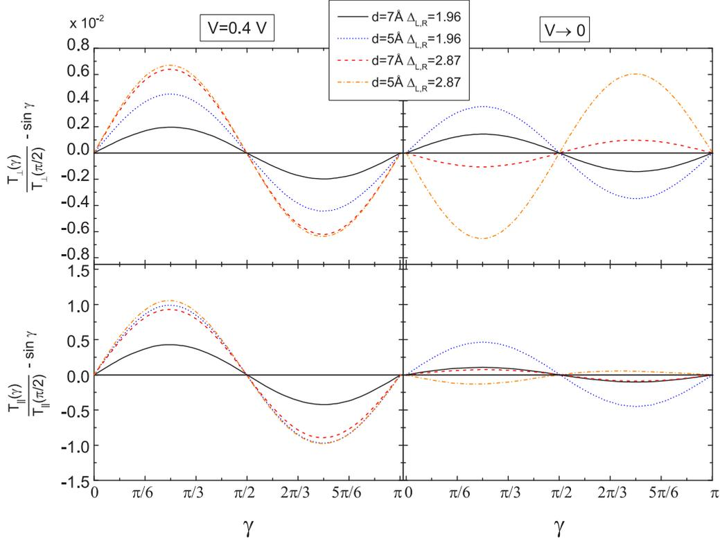
FIG. 3. (Color online) Angular dependence of a universal deviation function given by Eq. (7) for  $T_{\perp}$  (top panels) and  $T_{\parallel}$  (bottom panels) for different values of thickness  $d$ , exchange splittings  $\Delta_{L,R}$ , and applied voltages  $V$ . The parameters are  $\Delta_0 = 2.62$  eV,  $U_B = 0.5$  eV,  $m_{\text{eff}} = 0.4$ .
