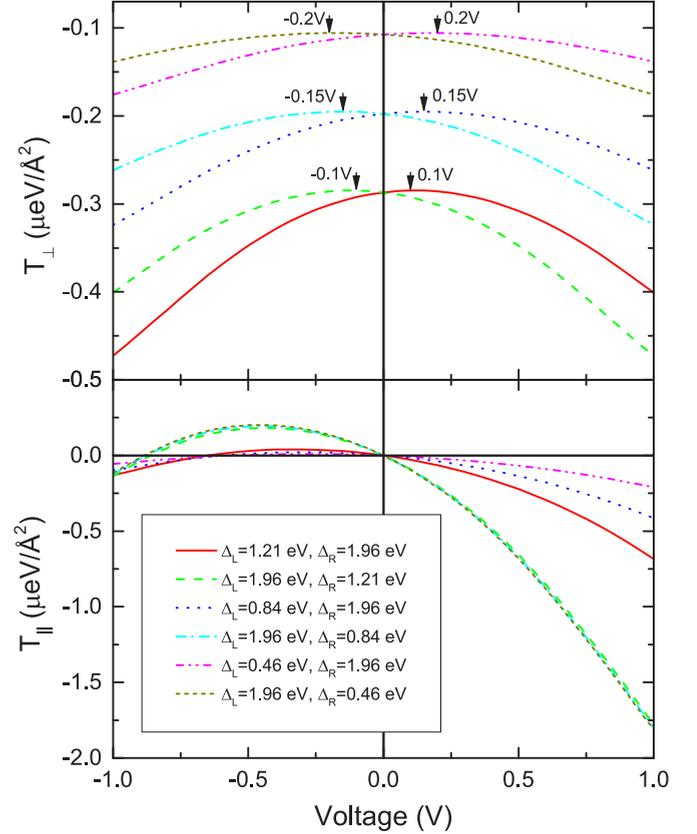
FIG. 2. (Color online) The out-of-plane  $T_{\perp}$  and in-plane  $T_{\parallel}$  torques as a function of applied bias in an asymmetric MTJ.  $U_B = 1$  eV,  $\Delta_0 = 2.62$  eV,  $m_{\text{eff}} = 0.4$ ,  $\gamma = \pi/2$ ,  $d = 7$  Å.
