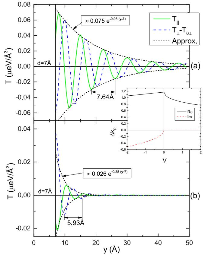
FIG. 5. (Color online) The same as in Fig. 4 for case in which the right FM electrode is a half-metal. Exchange splittings are  $\Delta_0 = \Delta_R = 2.62$  eV and  $\Delta_L = 1.96$  eV while other parameters are unchanged.
