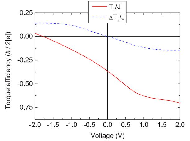
FIG. 6. (Color online) Bias voltage dependence of the torque efficiency for an MTJ.  $\Delta T_{\perp} = T_{\perp}(V) - T_{\perp}(0)$ . The parameters are  $\Delta_0 = 2.62$  eV,  $\Delta_L = \Delta_R = 1.96$  eV,  $U_B = 2$  eV,  $m_{\text{eff}} = 0.4$ ,  $\gamma = \pi/2$ ,  $d = 7$  Å.
