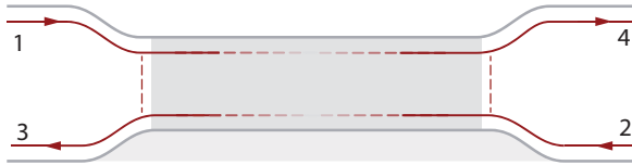
FIG. 2. (Color online) Schematic model of a quantum wire with two incoming (labeled 1 and 2) and two outgoing chiral modes (labeled 3 and 4) connecting to an extended scattering region. The dark shading represents a region of capacitive charging, the quantum dot. Near the entrance and exit to the quantum dot, where translational invariance is broken, backscattering of quasiparticles across the Hall bar is possible, denoted by vertical dashed lines. In a possible realization with a compressible quantum dot region, the edge current spreads into the bulk, and both elastic transmission along the edge (indicated by horizontal dashed line) and inelastic transmission through the dot is possible.
