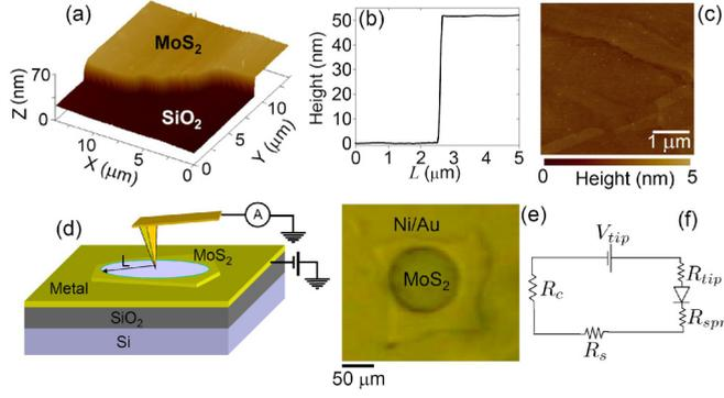
FIG. 1. (Color online) (a) AFM morphology of the edge of a multilayer MoS<sub>2</sub> flake and (b) corresponding height line profile, showing the thickness with respect to the SiO<sub>2</sub> substrate. (c) AFM image in the flake central area where CAFM measurements were performed. (d) Scheme of the experimental setup for CAFM measurements. (e) OM image of the fabricated test structure. (f) Circuitual schematic representation of the measured system.
