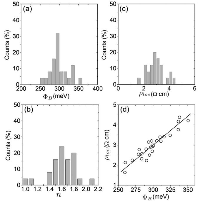
FIG. 3. Histograms of (a) the local SBH  $\Phi_B$ , (b) ideality factors  $n$ , and (c) resistivities  $\rho_{\text{loc}}$  extracted from the full set of  $I$ - $V_{\text{tip}}$  characteristics of Fig. 2(a). (d) Plot of  $\rho_{\text{loc}}$  vs  $\Phi_B$ .
