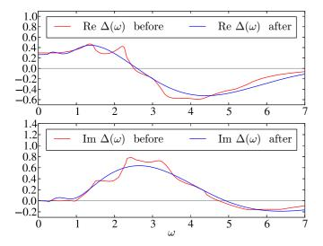
FIG. 2. (Color online) Red solid lines: spline interpolations of the real and imaginary parts of the gap function extracted from Ref. [10], before performing the maximum-entropy analytic continuation. Blue solid lines: real and imaginary parts of the gap function obtained from Eq. (13), after performing the maximum-entropy analytic continuation.
