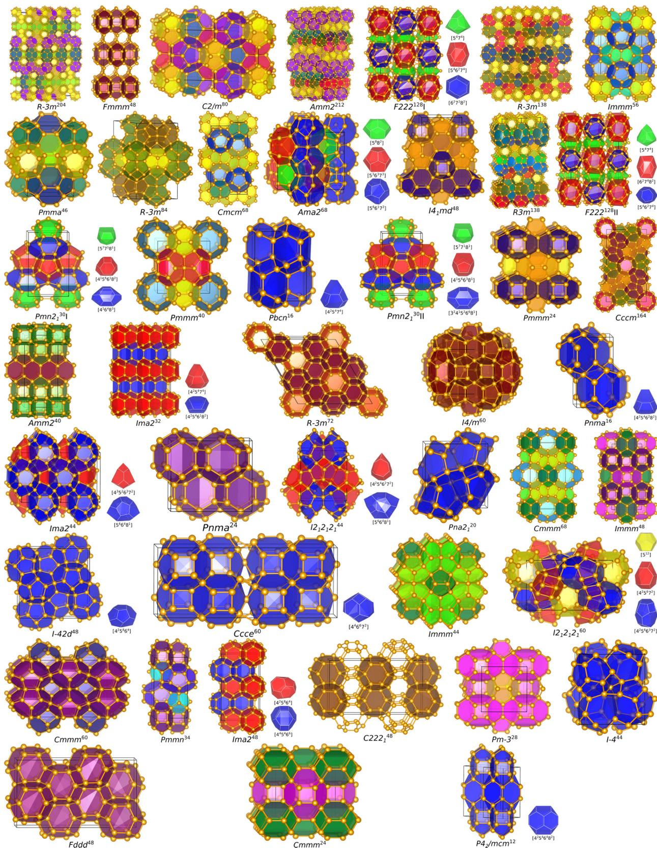
FIG. 3. (Color online) Low-density silicon allotropes formed of cagelike building blocks. The colors of the polyhedra correspond to the ones in Fig. 2.
