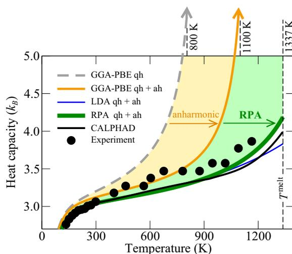
FIG. 1. (Color online) Ambient pressure heat capacity of Au ( $k_B$  = Boltzmann constant) utilizing various theory levels (qh = quasiharmonic, ah = anharmonic) and compared to experimental [20] and CALPHAD data [Scientific Group Thermodata Europe (SGTE) [21]] ( $T^{\text{melt}} = 1337$  K).
