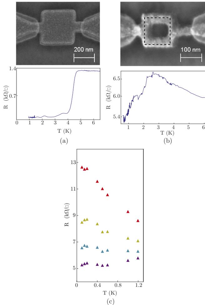
FIG. 1. (Color online) SEM image and  $R_{\square}$  vs  $T$  at  $B = 0$  T for (a) the disk and (b) the ring. The number of squares for such a ring (five squares) has been estimated from the geometry of the ring. The dashed line in (b) is the trajectory of a particle of a charge  $2e$ . (c)  $R$  vs  $T$  for the ring at  $B = 0, 0.7, 1.5, 4.0$  T (from bottom to top) showing the shift to insulating behavior.
