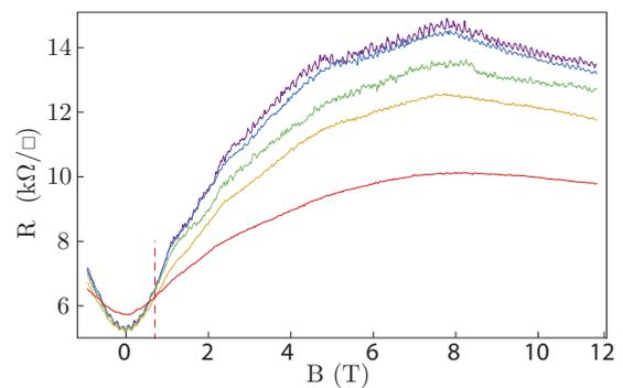
FIG. 2. (Color online)  $R$  vs  $B$  for temperatures  $T = 0.1, 0.2, 0.4, 0.6, 1.2$  K (from top to bottom at  $B = 8$  T), and the crossing point  $B_c \sim 0.8$  T is shown by the red dashed line.
