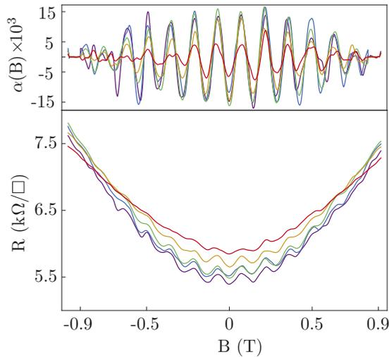
FIG. 3. (Color online)  $R$  vs  $B$  for the temperatures  $T = 0.15, 0.2, 0.5, 0.8$  K (from bottom to top at  $B = 0$  T); the inset: oscillating part  $\alpha(B)$  (see the text).
