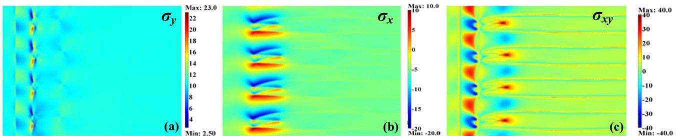
FIG. 3. (Color online) Stationary stress fields (in GPa) for  $K_{12} = 1.5 \times 10^{12} \text{ J/m}^3$ .
