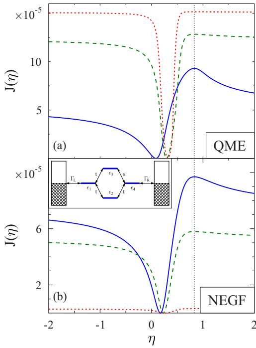
FIG. 4. (Color online) Efficiency LDF for a donor-bridge-acceptor junction calculated within the (a) QME and (b) NEGF approaches. Results are shown for constructive interference ( $s = t$ ; solid line, blue), single path ( $s = 0$ ; dashed line, green), and destructive interference ( $s = -0.8t$ ; dotted line, red). The vertical dashed line shows the Carnot efficiency. Other parameters are as in Fig. 3.
