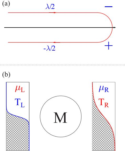
FIG. 1. (Color online) (a) Sketch of the counting field  $\lambda$  dressing the Keldysh contour forward ( $-$ ) and backward ( $+$ ) branches. (b) Sketch of a nano-thermoelectric junction consisting of a molecule  $M$  embedded between two contacts  $L$  and  $R$  with  $T_L < T_R$  and  $\mu_L > \mu_R$ .
