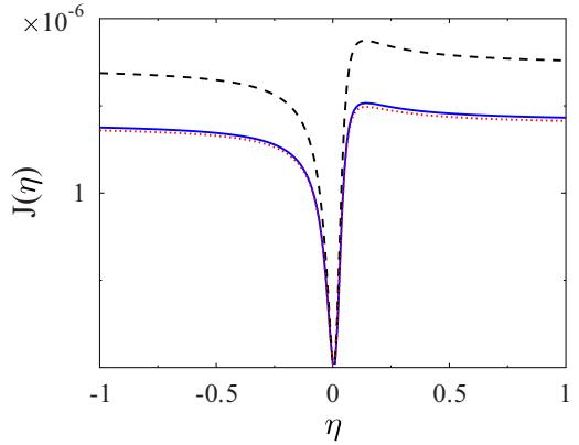
FIG. 6. (Color online) Efficiency LDF for a single-level junction (see inset in Fig. 5) calculated for experimentally relevant parameters. The predictions of the exact NEGF calculations (solid line, blue) are compared to the linear response predictions (29) (dashed line, black), and to the Gaussian approximation predictions (33) (dotted line, red). See text for parameters.
