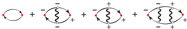
FIG. 6. (Color online) The simplest PSD approximation to the polarizability in terms of the screened interaction W (thick wiggly line).
