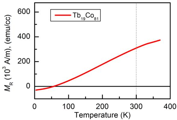
FIG. 8. (Color online) Remanent sample magnetization  $M_R$  versus temperature for a  $\text{Tb}_{19}\text{Co}_{81}$  amorphous alloy film of 20 nm thickness, measured by SQUID-VSM magnetometry in the temperature range  $T = 4\text{--}370$  K.  $M_R$  amounts to 300 kA/m (300 emu/cc) at room temperature and increases for rising temperatures.
