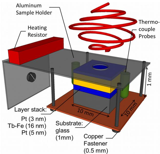
FIG. 1. (Color online) Heatable sample holder and layer stack. The sample is sandwiched between the heated aluminum top plate and a copper fastener. The heater is a 5-W, 330-m $\Omega$  heating resistor connected to an adjustable high-current power supply. To ensure proper heat conduction between the sample holder and the sample, it is embedded into a conductive paste. The temperature close to the sample position is measured by two thermocouple probes located on opposite sides of the sample.
