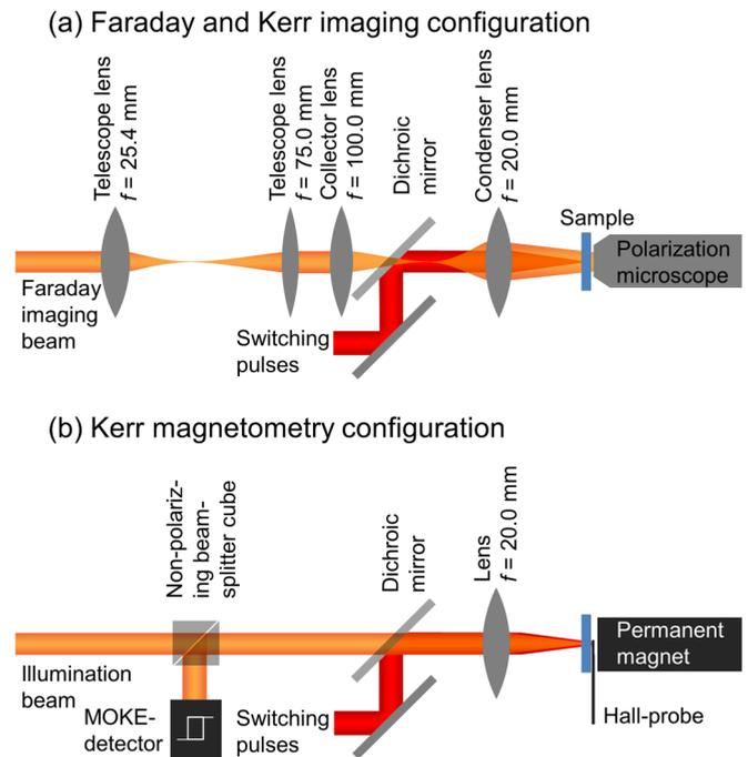
FIG. 2. (Color online) Beam geometry for (a) Faraday imaging and (b) Kerr magnetometry.
