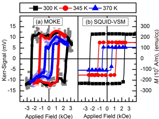
FIG. 5. (Color online) Hysteresis loops of Tb<sub>34</sub>Fe<sub>66</sub> at various sample temperatures of  $T = 300$ , 345, and 370 K, measured by a MOKE and by SQUID-VSM. For elevated sample temperatures the coercivity as well as the remanence decreases, which facilitates AOS at a pulse repetition rate of  $\nu = 10$  kHz at  $T = 370$  K.
