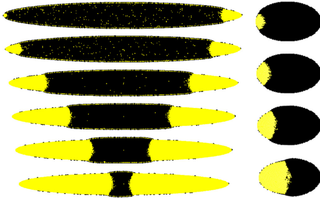
FIG. 3. (Color online) Left: Most probable cluster evolution at T = 100 K for highly elongated ellipses (high eccentricities; in this case the ellipses are composed of 46 969 molecules, with the ratio 10 between the major and minor axes of the ellipses and 720 molecules on the major axis). The two clusters join somewhere near the middle of the ellipse. Right: Possible spreading of one single cluster for smaller ellipses (in the figure the ellipses are composed of 4545 molecules, with the ratio 2 between axes and 100 molecules on the major axis).
