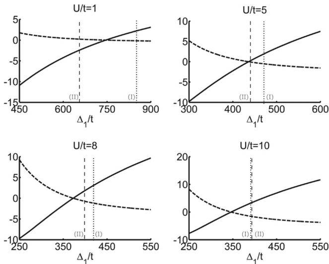
FIG. 2.  $\delta$  (solid lines) and  $\eta$  (dashed lines) as functions of  $\Delta_1$  for  $U/t = 1, 5, 8, 10$  and  $g_q = 120 \text{ MHz} \times 2\pi$ . As Eq. (16) shows,  $\delta$  and  $\eta$  are the displacements of the on-site energy and on-site interaction of the first site. The vertical lines labeled (I) and (II) indicate the mean-field critical values of the two cases discussed in Sec. III.
