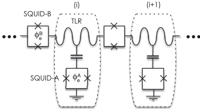
FIG. 1. Schematic plot of the 1D TLR array. SQUID A, as a tunable charge qubit, is capacitively coupled to the center of a TLR. Nearest-neighbor sites are connected by SQUID B. The external magnetic fluxes  $\phi_e^A$  and  $\phi_e^B$  through SQUIDS A and B can be used to tune their Josephson energies.
