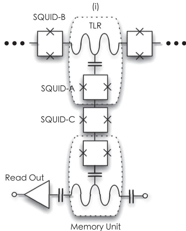
FIG. 9. Measuring the photons in the simulator: Each site of the simulator is connected to a memory unit formed by another qubit-TLR system via a tunable SQUID (labeled SQUID C) acting as a switch. Measurements of the photon number in the memory unit can be applied [76–78]. This memory unit can also serve as a circuit for preparing the initial state by manipulating SQUID C and SQUID B.
