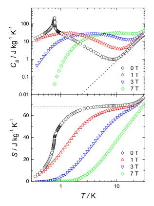
FIG. 4. (Color online) Top: Heat capacity at applied magnetic field  $C_B(T)$ . Dashed line: Calculation of the phonon contribution. Bottom: Entropy S(T, B) deduced from heat capacity. Details in the text. Dotted line: infinite temperature limit for the molar magnetic entropy  $S_m/R(\infty) = \ln(2s+1)$  for s = 7/2.
