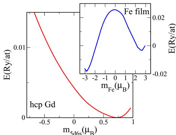
FIG. 1. (Color online) Energy of hcp Gd as a function of the value of spin moment of  $5d6s$  electrons. In the inset the energy of the fcc Fe film as the function of the moment of the atoms of the first layer.
