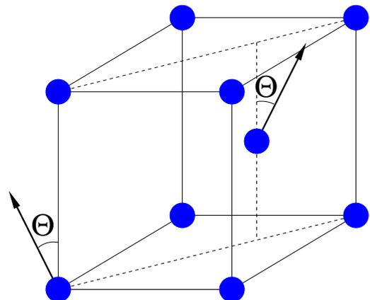
FIG. 2. (Color online) The unit cell of the hcp structure. The arrows show the directions of the  $4f$  spin moments for two Gd atoms in the unit cell. The atoms connected by lattice translations have the same directions of the spin moments.
