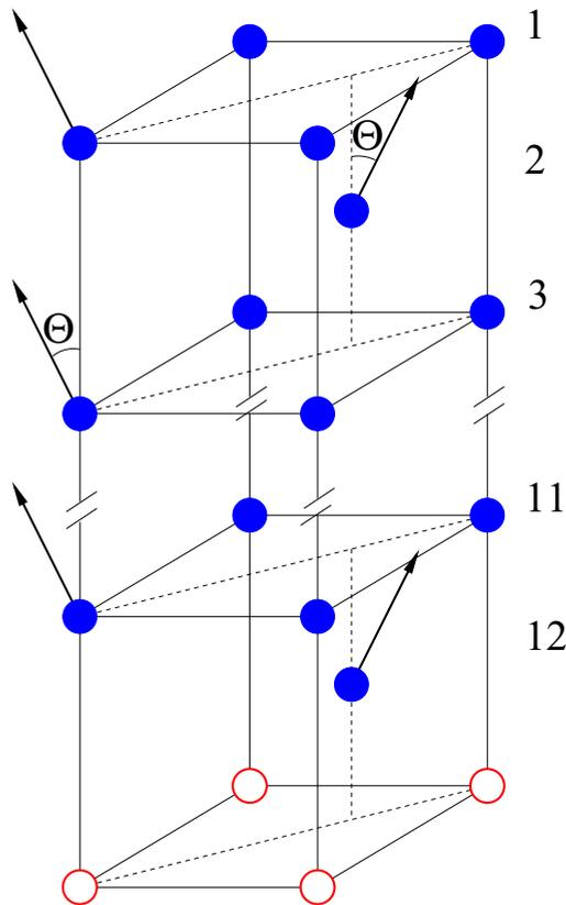
FIG. 7. (Color online) The slab unit cell. Most of the results presented in the paper are obtained for 12 Gd layers and 4 layers of the empty spheres. The arrows show the directions of the atomic  $4f$  moments. The empty red circles show the first layer of the empty spheres. The atoms belonging to the same plane have the same direction of the spin moments.
