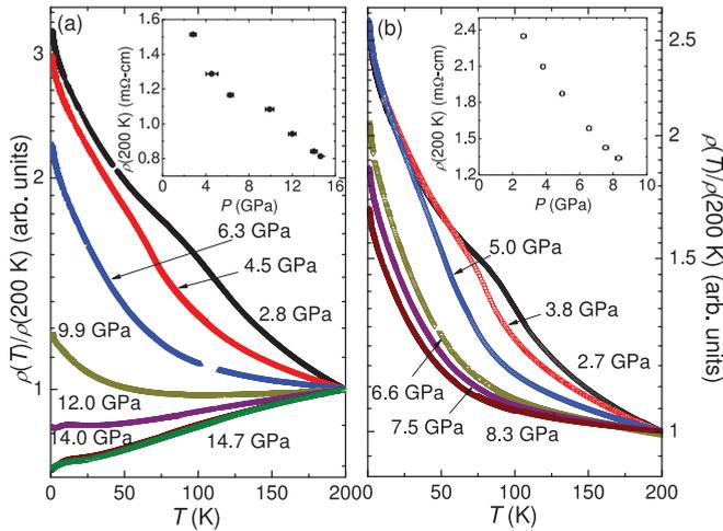
FIG. 2. (Color online) Electrical resistivity  $\rho$  vs temperature  $T$  on a semilog scale for two distinct samples of LaFeAsO using the Bridgman anvil cell technique from 2.7 to 14.7 GPa. The data have been normalized by their value at 200 K. The inset in each panel shows the electrical resistivity values at 200 K for each pressure.
