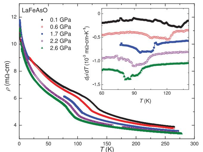
FIG. 1. (Color online) Electrical resistivity  $\rho$  vs temperature  $T$  measured in quasihydrostatic applied pressures up to 2.6 GPa. Spin-density wave order is suppressed with increasing pressure from approximately 134 to 80 K. The inset shows the first derivative of the electrical resistivity with respect to temperature with each set of data offset by a constant value.
