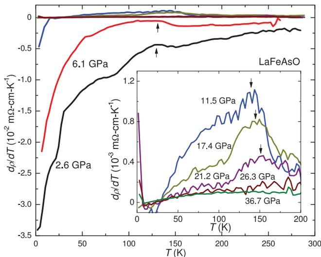
FIG. 5. (Color online) The first derivative of the electrical resistivity  $\rho$  with respect to temperature  $T$ ,  $d\rho/dT$  vs  $T$ , measured in a diamond anvil cell. The  $d\rho/dT$  data reveal a feature corresponding to spin-density wave order as well as an unexpected feature at higher temperature  $T^*$ . The inset emphasizes the feature at  $T^*$  in the data measured under applied pressures from 11.5 to 36.7 GPa. It is clear that  $T^*$  increases with increasing pressure.
