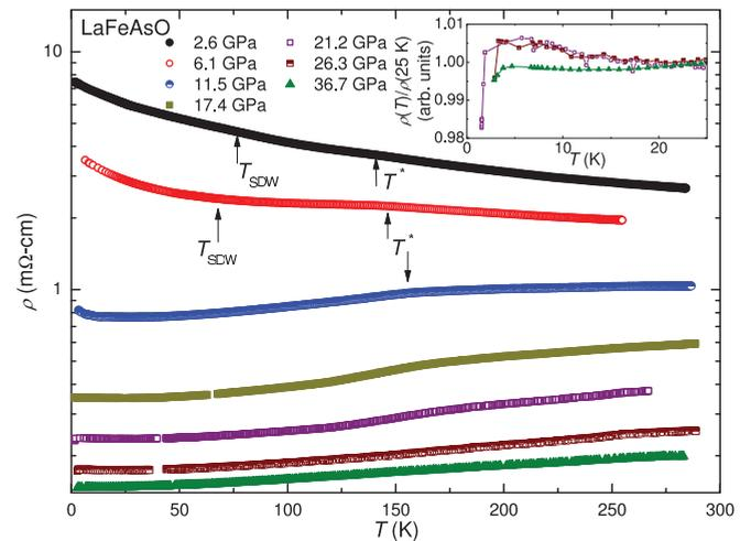
FIG. 4. (Color online) Electrical resistivity  $\rho$  vs temperature  $T$  measured using a diamond anvil cell from 2.6 to 36.7 GPa. A metallic state is clearly induced near 11.5 GPa. We also note the evolution of a high-temperature feature at a temperature denoted as  $T^*$ . The inset shows  $\rho(T)$  data normalized to their values at 25 K for measurements under applied pressure  $P \geq 21.2$  GPa. A sharp low-temperature downturn is observed in each case.
