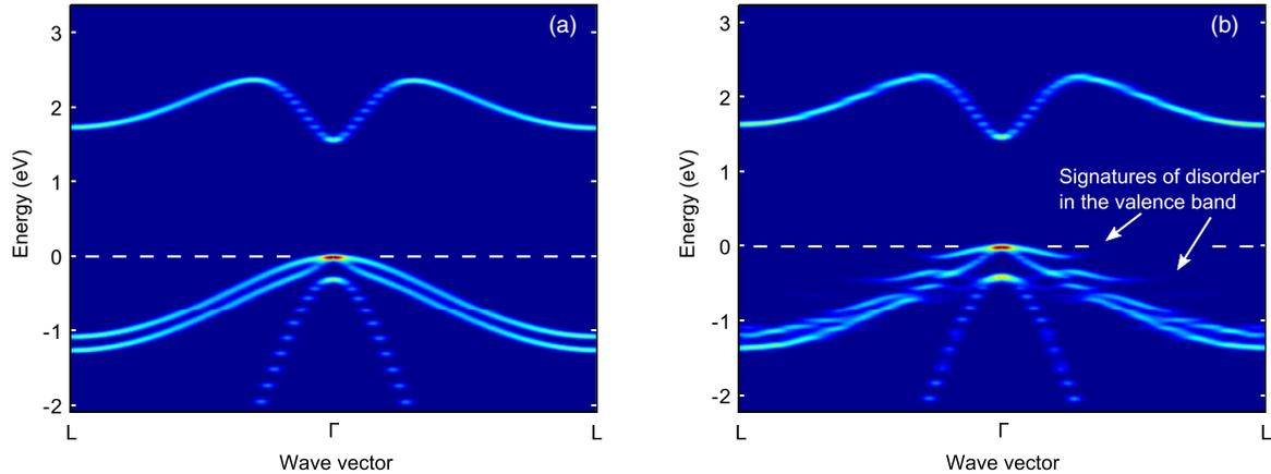
FIG. 4. (Color online) Band structure of  $\text{Ga}_{64}\text{As}_{64}$  (a) and  $\text{Ga}_{64}\text{As}_{63}\text{Bi}_1$  (b) supercells unfolded to the primitive Bloch representation. Bismuth incorporation leads to perturbations in the valence band, reduction of the band gap, and enhanced spin-orbit splitting.
