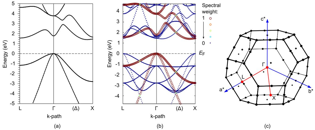
FIG. 2. (Color online) Band structure of GaP: 2-atom primitive unit cell (a) and 16-atom  $2 \times 2 \times 2$  supercell (b). The supercell band structure is “obfuscated” due to the zone folding. Fat bands on panel (b) illustrate the unfolded band structure where the symbols size and color represent the Bloch spectral weight. Both cells have the Brillouin zone shown on panel (c). Here and in all figures hereafter the Fermi energy is set to zero.
