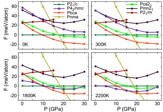
FIG. 2. (Color online) Free energies  $F$  calculated at  $T = 0$  K,  $T = 300$  K,  $T = 1800$  K, and  $T = 2200$  K for the identified low-energy phases of hafnia and shown as functions of pressure  $P$ . Data is given by symbols while curves are guides to the eye. Data corresponding to the  $Pm$ ,  $Cc$ , and  $P1$  phases are not shown as they are energetically unfavorable by roughly 250 meV/atom compared with the other phases.
