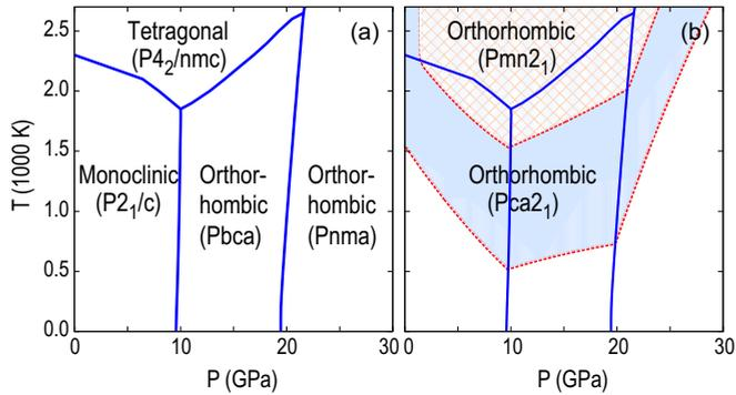
FIG. 1. (Color online) (a) Computed equilibrium phase diagram of hafnia and (b) regimes in which  $\Delta F(P, T)$ , the free energy difference between  $Pca2_1$  and  $Pmn2_1$  phases, and the equilibrium phases are small, i.e.,  $\Delta F(P, T) < k_B T/5$ .
