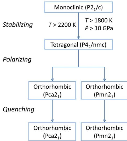
FIG. 5. (Color online) Possible pathways which might describe the formation process of hafnia polar phases. First, the  $P4_2/nmc$  tetragonal phase is stabilized at suitable temperature and/or pressure. Next, this phase may be driven into a polar phase in the subsequent polarizing step. Finally, the polar phase may be quenched to lower temperatures and pressures.
